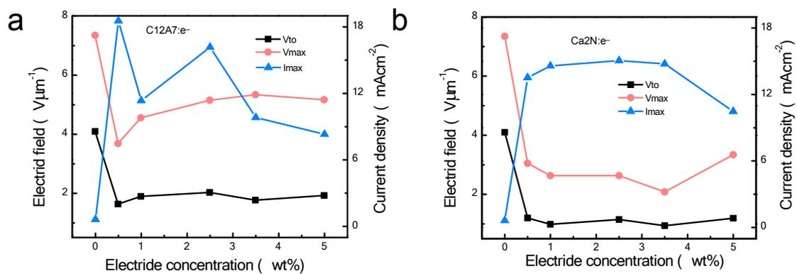
**Figure S8.** Comparison of the turn on voltage ( $V_{to}$ ), maximum current density ( $I_{max}$ ), and the electric field at maximum current density ( $V_{max}$ ). a) C12A7:e<sup>-</sup>-PSWNT-Ag pastes. b) Ca2N:e<sup>-</sup>-PSWNT-Ag pastes.
