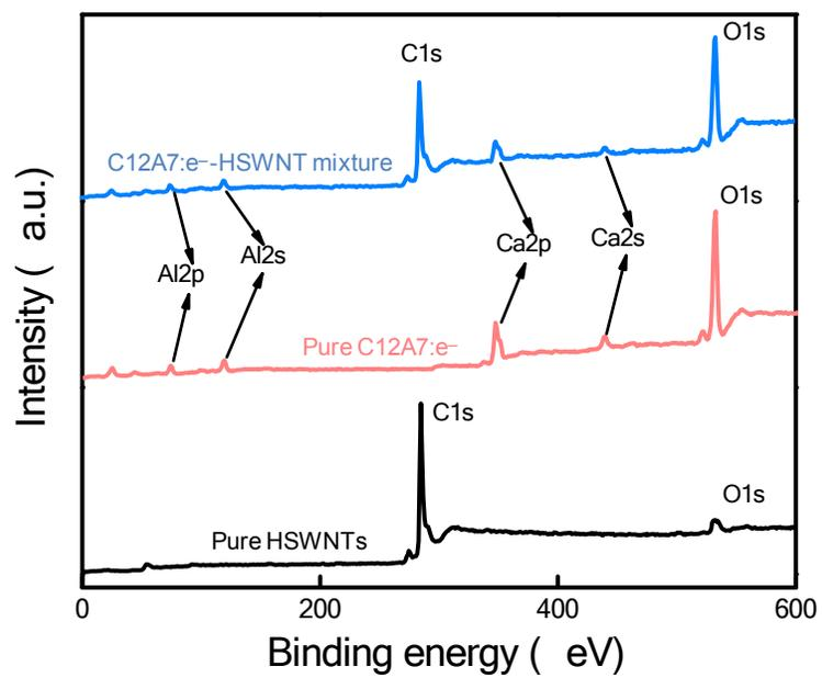
**Figure S2.** Wide scan XPS data of pure HSWNTs, pure C12A7:e<sup>-</sup> powder, and C12A7:e<sup>-</sup>-HSWNT powder mixture (50:50 wt.%).
