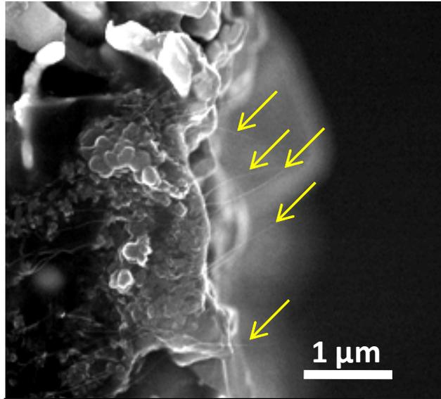
**Figure S7.** Cross-sectional SEM image of the tape-activated PSWNT-Ag paste. The surface was activated 10 times using Scotch tapes.<sup>S6</sup> The yellow arrows indicate nanotubes.
