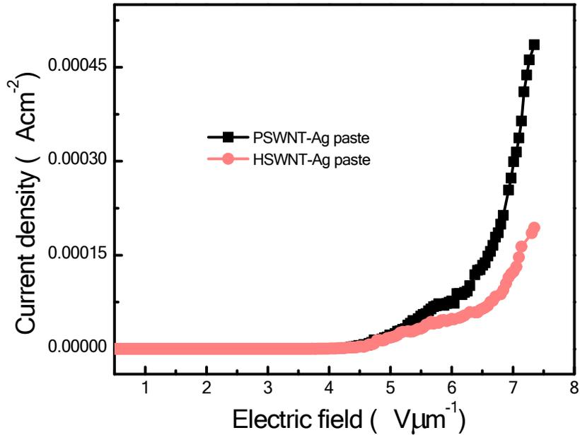
**Figure S1.** Field emission characteristics of the PSWNT-Ag paste and HSWNT-Ag paste. The nanotubes were mixed with Ag pastes without electrified particles. The nanotube, silver, and epoxy concentrations were 2.5, 80, and 17.5 wt.%. The field emission current density of PSWNT-Ag paste was 0.48 mA/cm<sup>2</sup> at 7.3 V/μm with a turn on voltage of 4.14 V/μm. The field emission current density of HSWNT-Ag paste was 0.19 mA/cm<sup>2</sup> at 7.34 V/μm with a turn on voltage of 4.2 V/μm.
