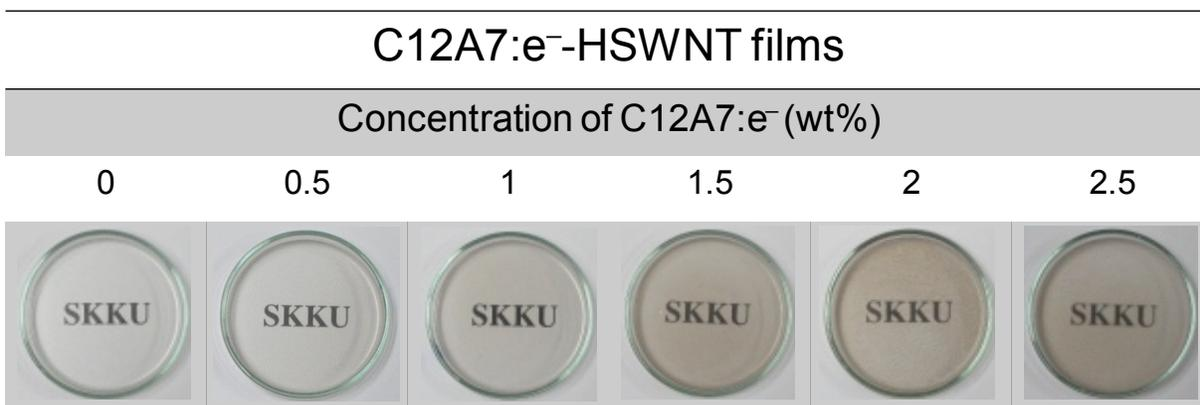
**Figure S5.** Optical images of C12A7:e<sup>-</sup>-HSWNT films. The letters SKKU are placed behind the films. The transmittance decreased from 84.8 % to 30 % at 550 nm with the addition of 0 to 2.5 wt.% C12A7:e<sup>-</sup> particles.
