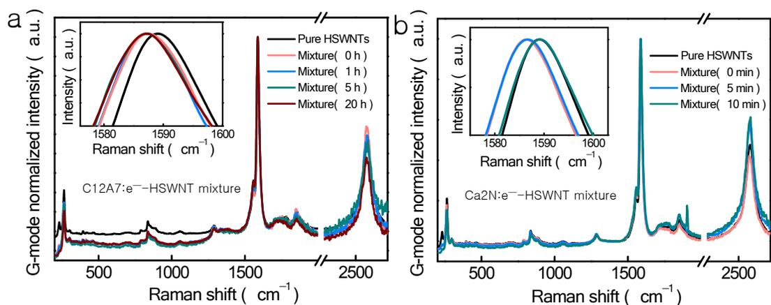
**Figure S4.** Raman spectra of pure HSWNTs and electrified-HSWNT powder mixtures. The time after exposure of the powder mixtures to air is shown in parenthesis. The G-mode shift is magnified in the inset. a) C12A7:e<sup>-</sup>-HSWNT powder mixture. b) Ca2N:e<sup>-</sup>-HSWNT powder mixture.
