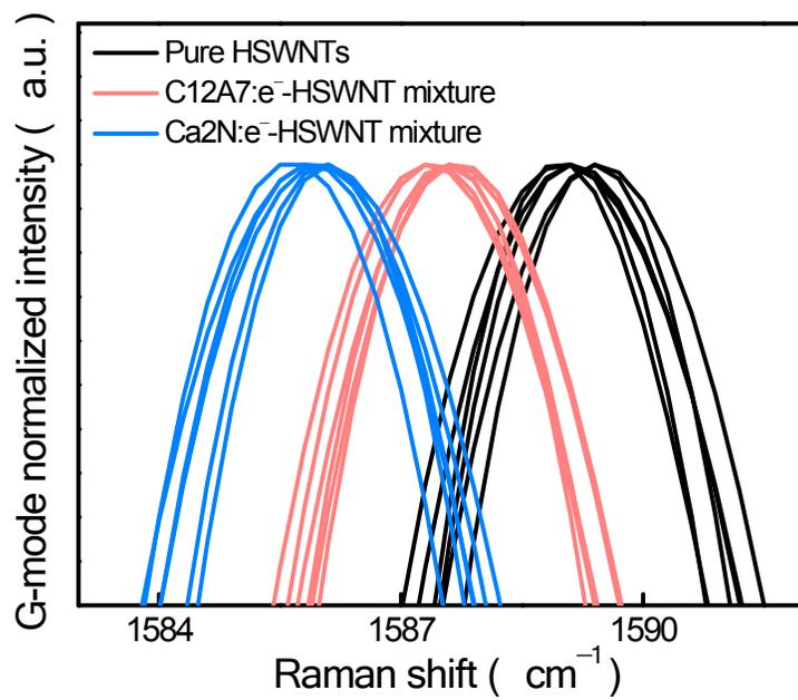
**Figure S3.** The G-mode of Raman spectra measured at 6 different locations in pure HSWNTs, C12A7:e<sup>-</sup>-HSWNT, and Ca2N:e<sup>-</sup>-HSWNT powder mixtures.
