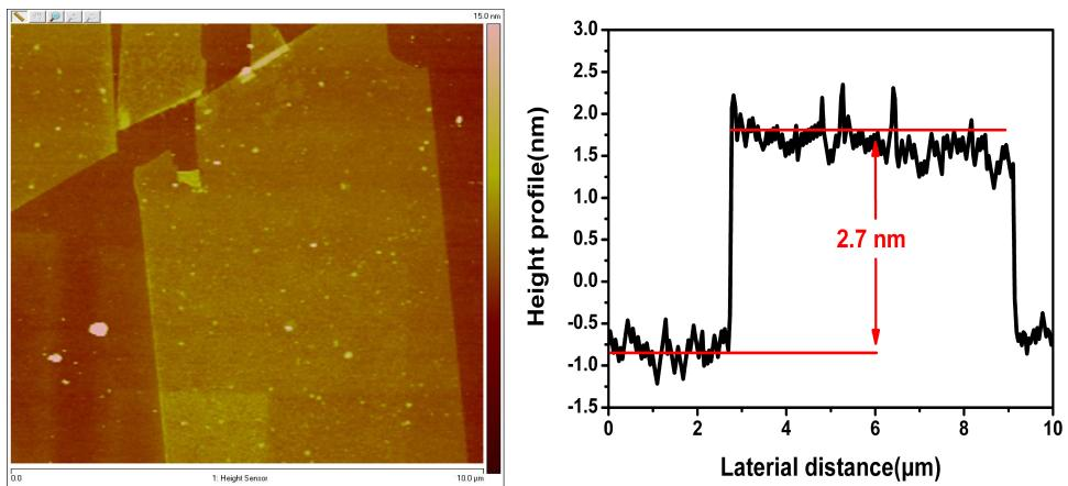
**Figure S2. AFM height image of few-layer  $\text{ReSe}_2$ .**
