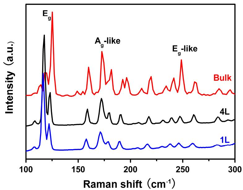
**Figure S3.** Raman spectra of ReSe<sub>2</sub> nanosheets.
