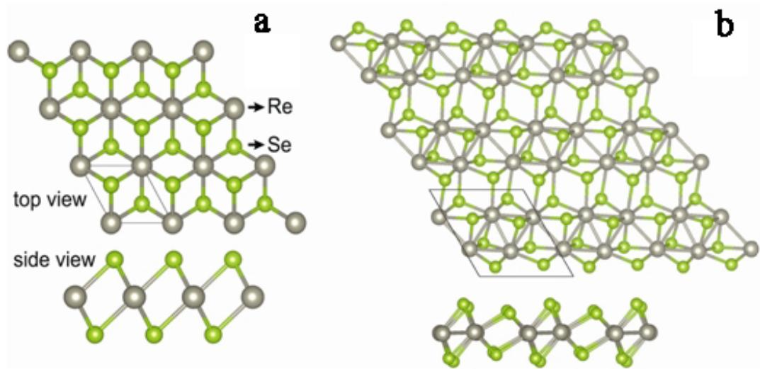
**Figure S1. The structure of ReSe<sub>2</sub>.** **a.** Undistorted ReSe<sub>2</sub>, **b.** distorted ReSe<sub>2</sub>.
