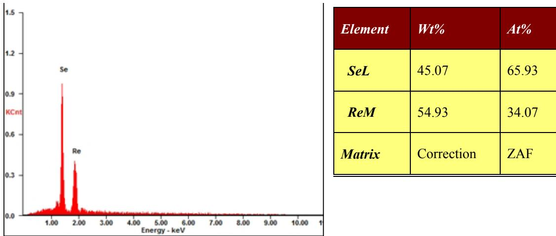
**Figure S5. EDX of  $\text{ReSe}_2$  nanosheet.**
