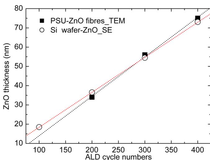
**Figure S2.** The thickness of ZnO as a function of ALD cycle numbers for two contexts, namely, PSU-ZnO fibers and ZnO coating on silicon wafer. The former case is from TEM image analysis, while the latter from spectroscopic ellipsometry (SE).
