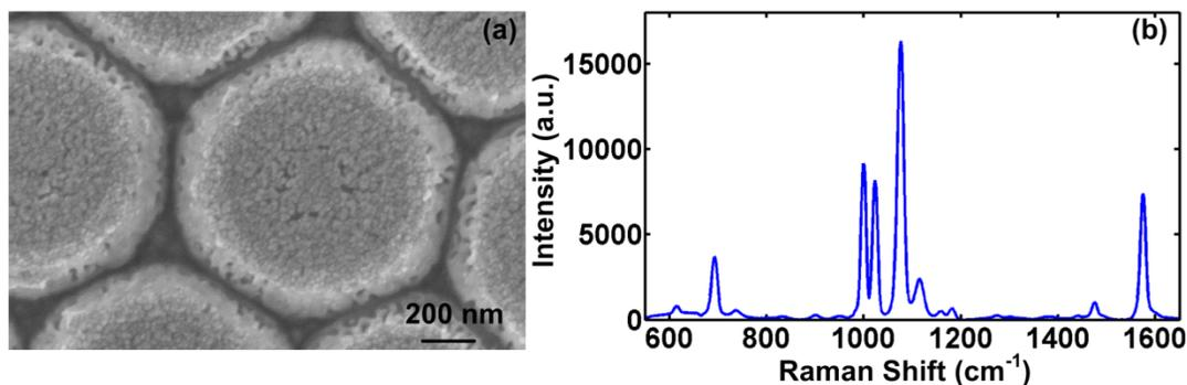
Figure. S1. (a) Scanning electron micrograph of NPG disks; (b) average SERS spectrum from a single NPG disk.
