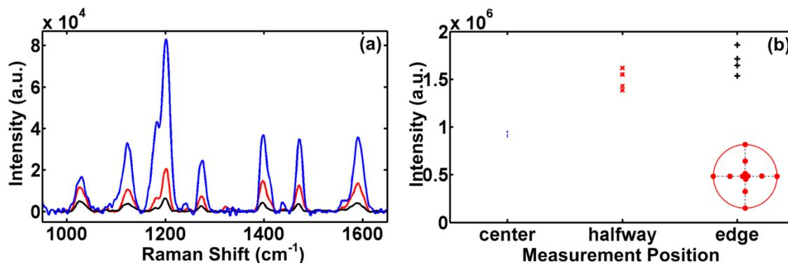
Figure. S2. (a) averaged SERS spectra before (blue), after (red) MCH treatment and after buffer wash step (black); (b) Cy3 SERS intensities at different physical positions, the red circle represents the dried area of probe solution, and the red dots represent measurement positions.
