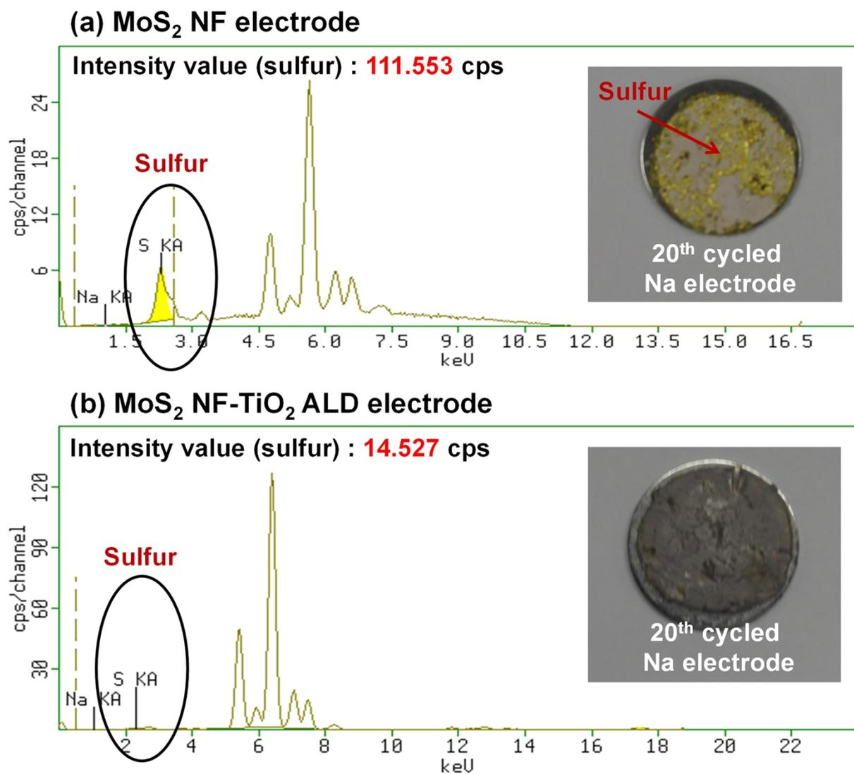
**Figure S7.** *Ex-situ* X-ray fluorescence analysis of the MoS<sub>2</sub> NF electrode and the TiO<sub>2</sub>-coated MoS<sub>2</sub> NF electrode collected after the 20<sup>th</sup> cycle. The inset figures are *ex-situ* SEM images of a sodium metal electrode loaded onto a stainless steel spacer in a 2032 coin cell.
