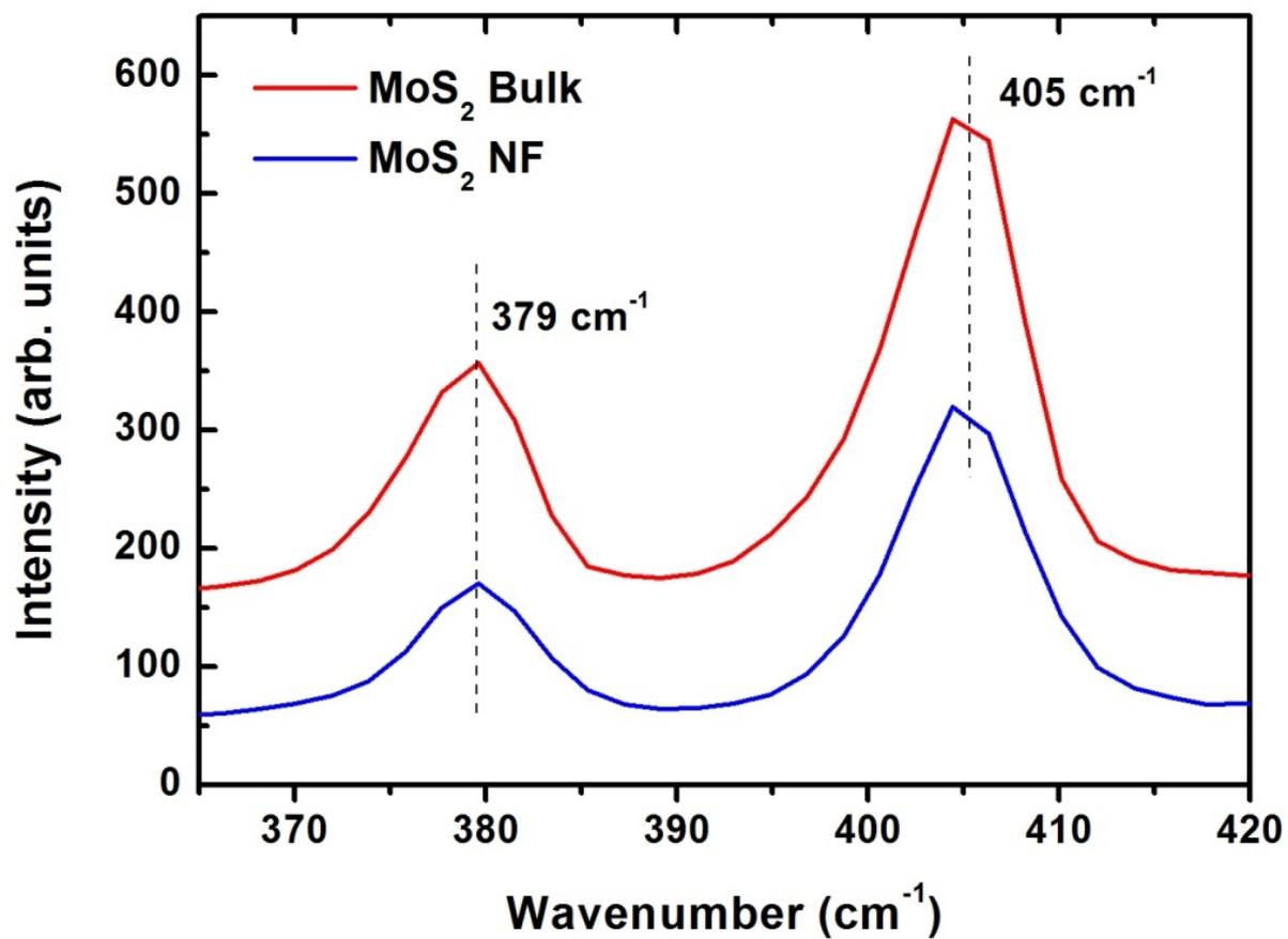
**Figure S2.** Raman spectra obtained from the bulk MoS<sub>2</sub> and the MoS<sub>2</sub> NFs corresponding to the Mo-S vibration mode
