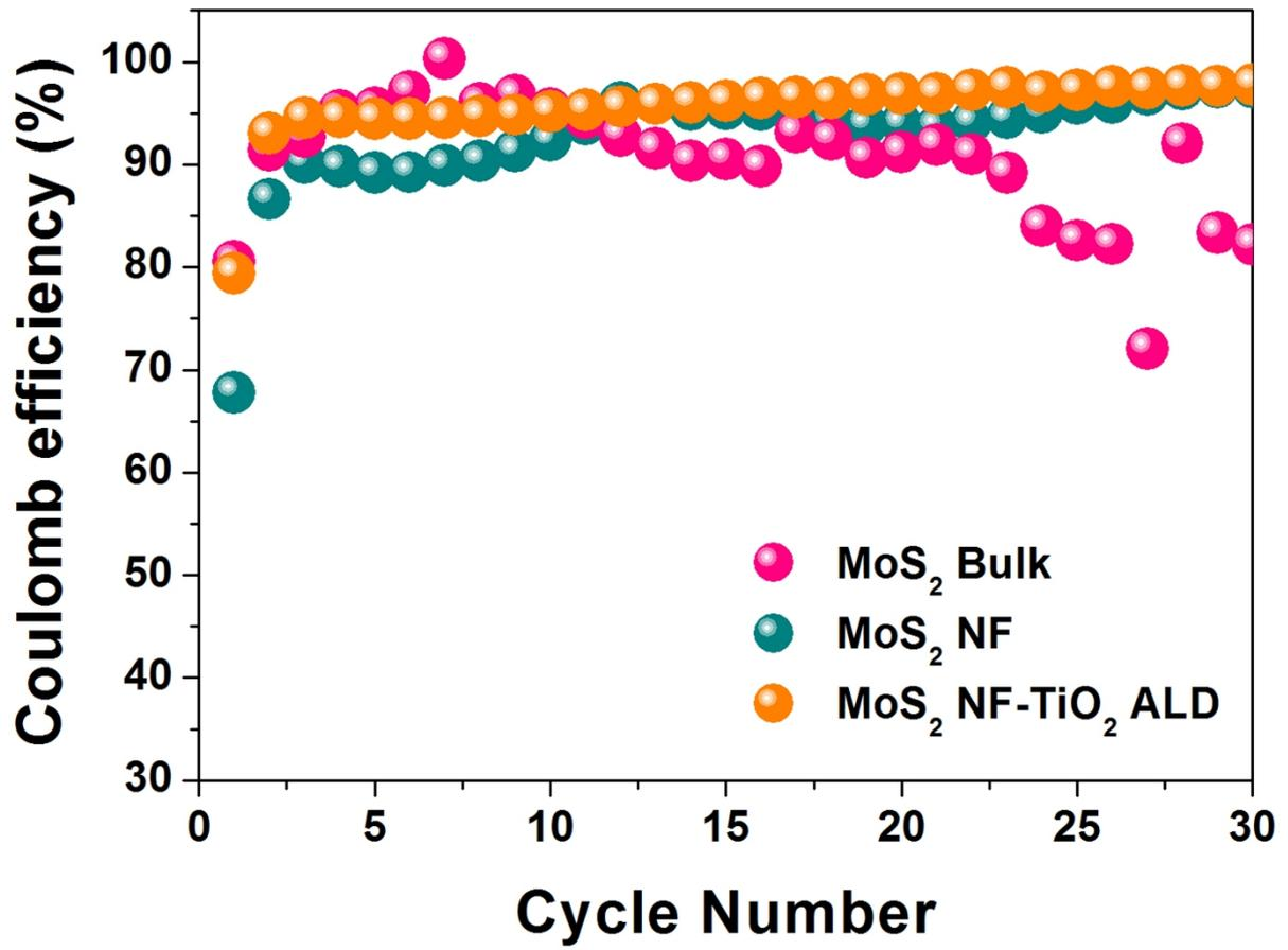
**Figure S6.** Coulomb efficiencies of the bulk MoS<sub>2</sub> electrode, the MoS<sub>2</sub> NF electrode, and the TiO<sub>2</sub>-coated MoS<sub>2</sub> NF electrode during charge/discharge cycling in a voltage window between 3.0 and 0.01 V at a current density of 100 mA/g.
