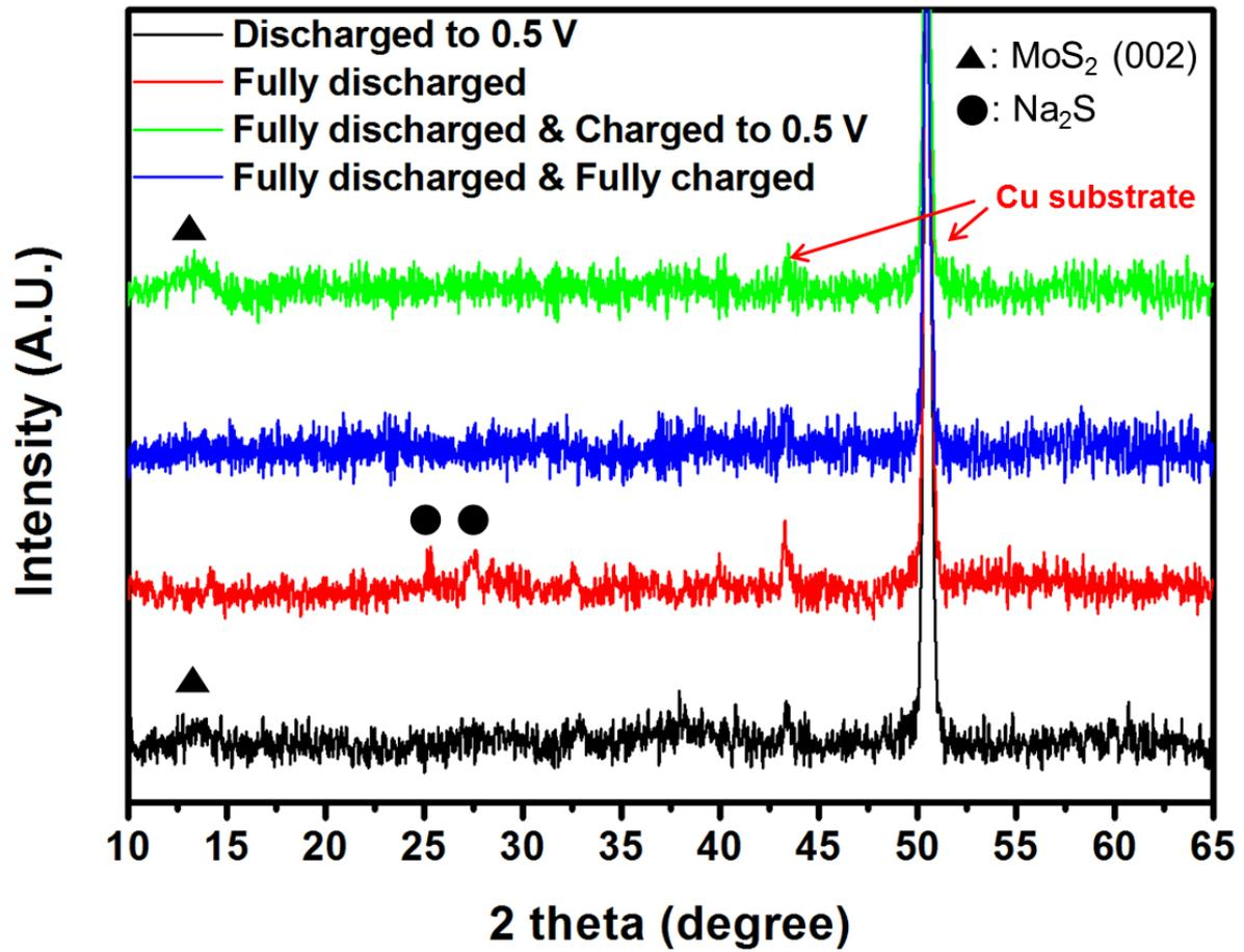
**Figure S4.** *Ex-situ* X-ray diffraction patterns of the MoS<sub>2</sub> NFs collected at various states during the charge and discharge process
