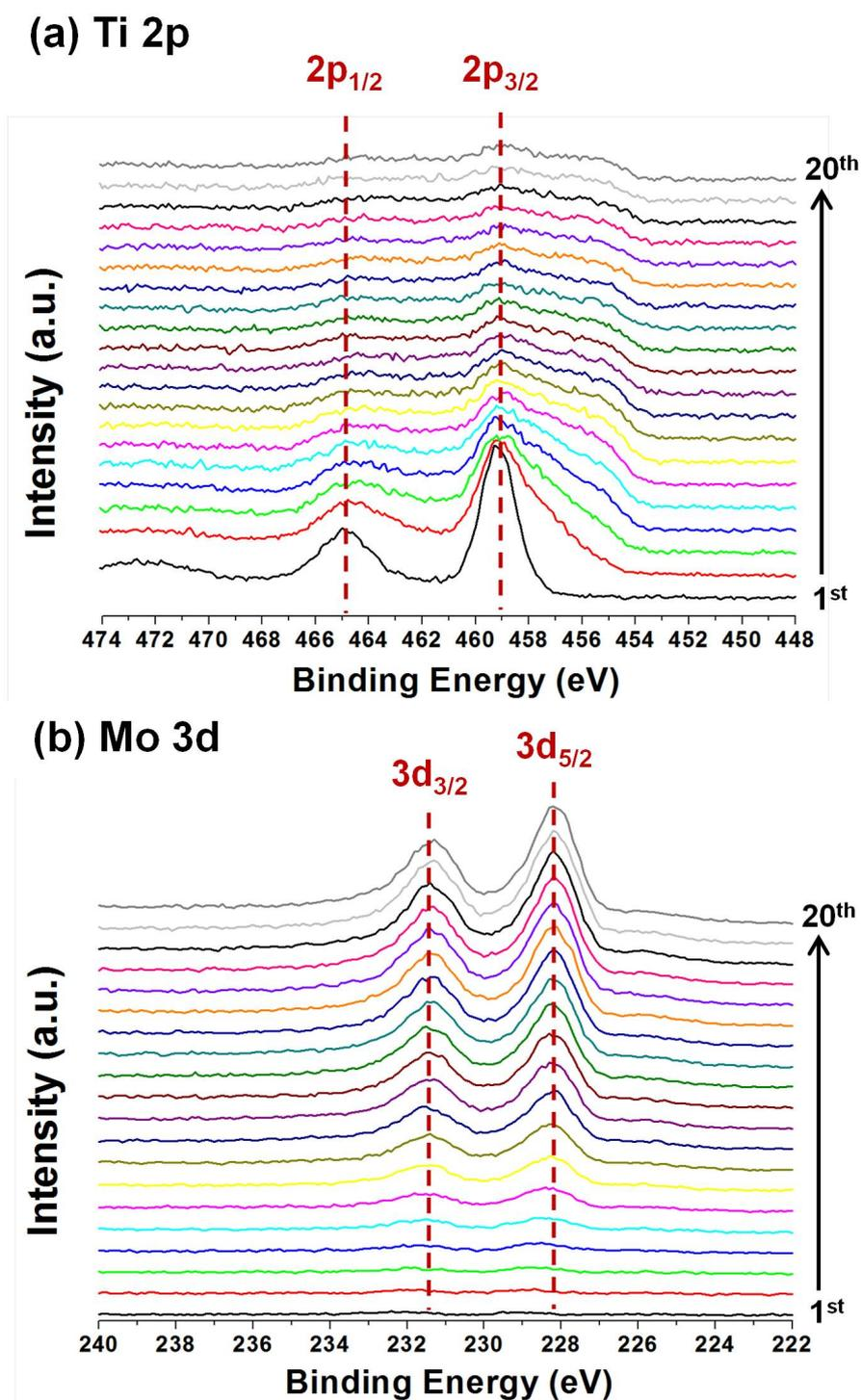
**Figure S5.** X-ray photoelectron spectra collected in the (a) Ti 2p and (b) Mo 3d regions obtained from the TiO<sub>2</sub>-coated MoS<sub>2</sub> NF electrode. The XPS spectra of the electrodes were collected at a depth profile of 20 cycles.
