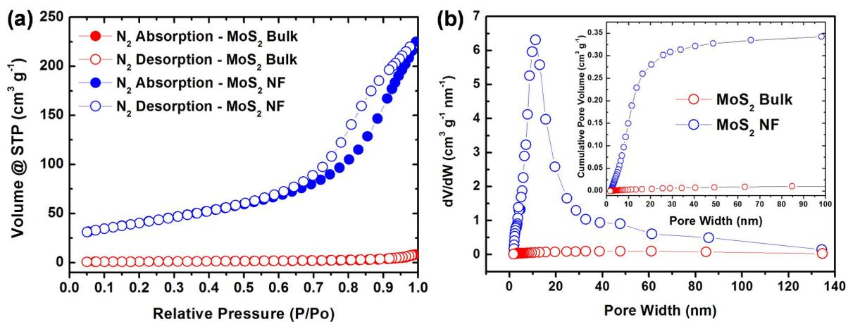
**Figure S3.** (a) Nitrogen adsorption/desorption isotherms obtained at 77 K, (b) pore size distribution, and cumulative pore volume (inset) of the bulk MoS<sub>2</sub> and the MoS<sub>2</sub> NFs
