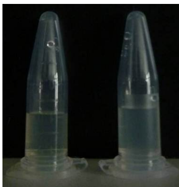
Fig. S1. Photos taken at 1 min after addition of \text{AgNO}_3 (final concentration: 1 mM) to mixture containing only 1 mM \text{AuCl}_4^- (left) or 1 mM \text{AuCl}_4^- and 2 mM cytidine (right). The right sample was cloudy while the left one kept clear.
