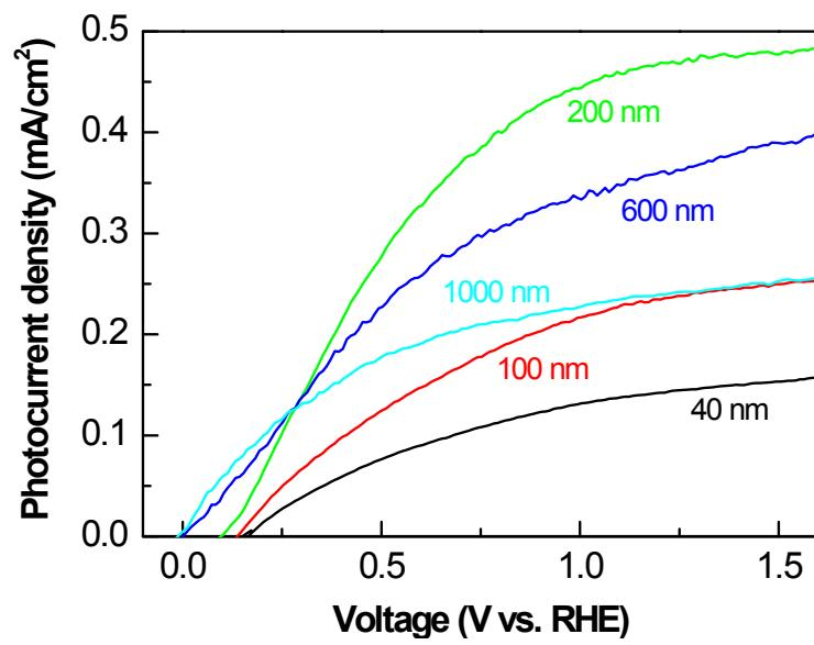
**Figure S7.**  $J$ - $V$  curves of the TiO<sub>2</sub> NP (P25) film-based photoelectrodes, under 100 mW/cm<sup>2</sup> (Xe lamp) of light illumination.
