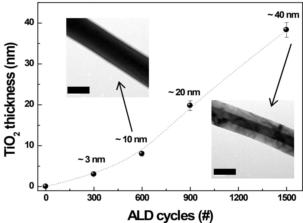
**Figure S5.** The thickness of the  $\text{TiO}_2$  nanoshell versus the number of ALD cycles. The insets show the TEM images of the  $\text{TiO}_2$  nanoshell coated ITO NW (scale bar: 100 nm).
