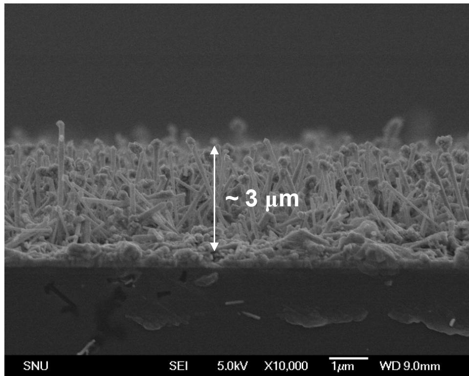
**Figure S4.** Cross-sectional SEM image of an ITO NW array grown without Au seeds for 30 min. All the other growth conditions are identical to the conditions for Au seed layer-mediated growth.
