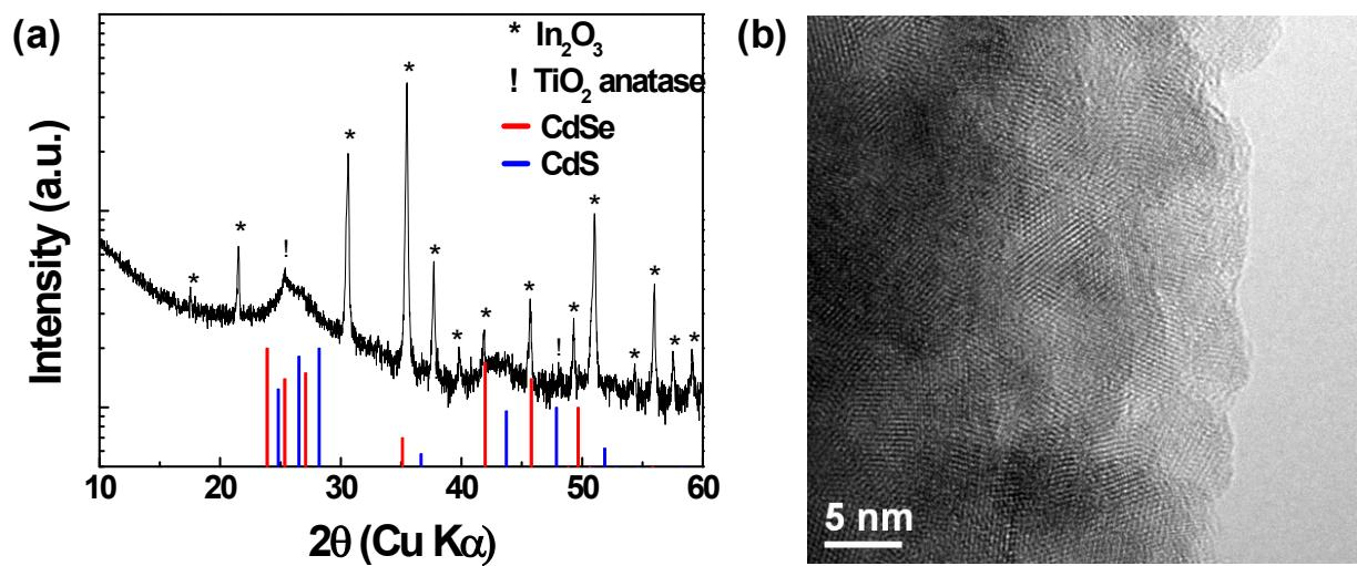
**Figure S9.** (a) XRD pattern and (b) HRTEM image of the CdS/CdSe crystallites coated on the surface of  $\text{TiO}_2$  nanoshell.
