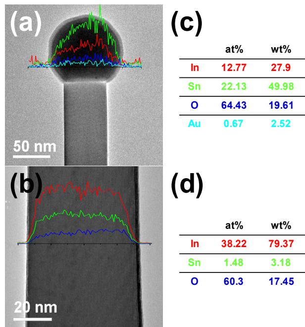
**Figure S3.** EDS line scan results (red: In, green: Sn, blue: O, and cyan: Au) of the (a) tip and (b) body of a NW, and the corresponding composition tables (c and d), respectively.
