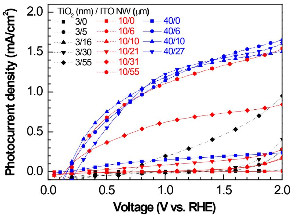
**Figure S6.** *J-V* curves of the TiO<sub>2</sub>/ITO NW-based photoelectrodes, under 100 mW/cm<sup>2</sup> (Xe lamp) of light illumination.
