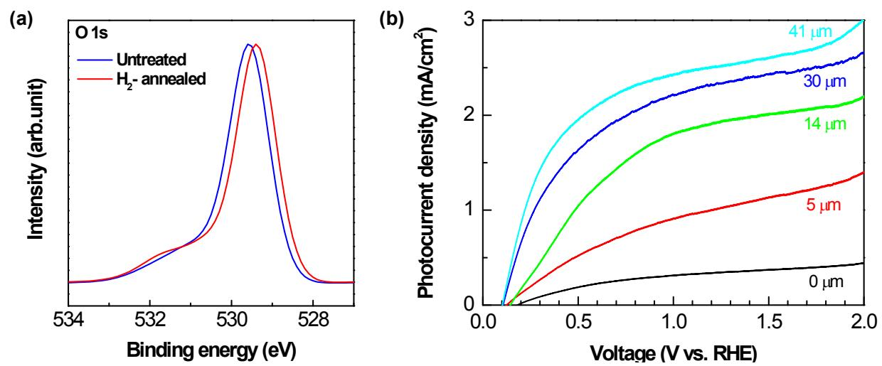
**Figure S8.** (a) O 1s XPS peaks of the ITO NW and (b)  $J$ - $V$  curves for the H<sub>2</sub>-annealed photoanodes (20 nm-thick TiO<sub>2</sub>/ITO NW).
