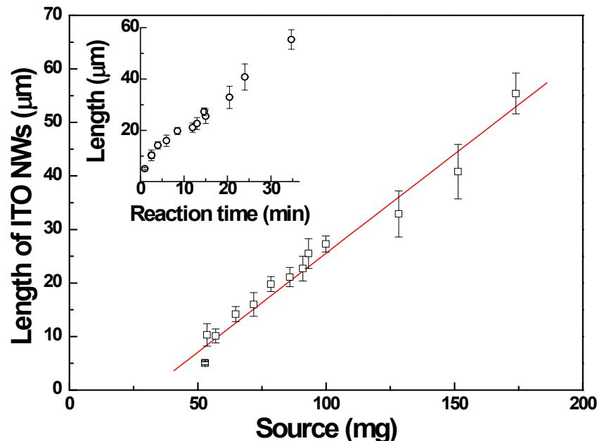
**Figure S1.** Length of the grown ITO NWs as a function of the consumed source amount. The x-intercept of the extrapolated line is attributed to a loss of source by evaporation during heating up to 600°C. Inset shows the length of ITO NWs as a function of reaction time.
