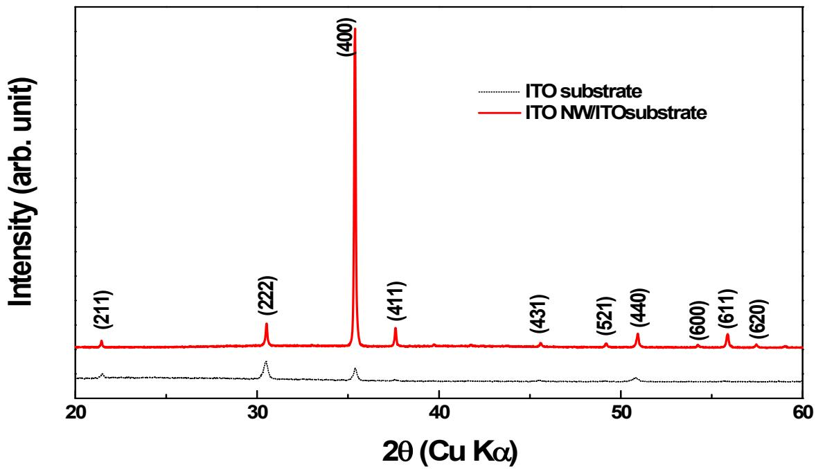
**Figure S2.** XRD pattern of the bare ITO substrate (ITO thin film on glass) and the grown NWs on the ITO substrate. All the peaks correspond to the peaks for cubic  $\text{In}_2\text{O}_3$  shown in JCPDS Card No. 06-0416.
