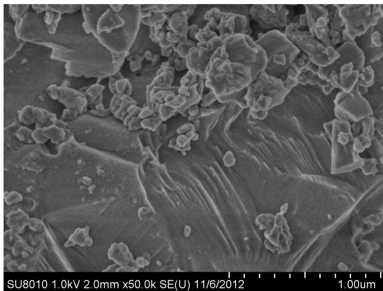
Figure S3. FESEM image of the Co-ZIF-9 catalyst.
