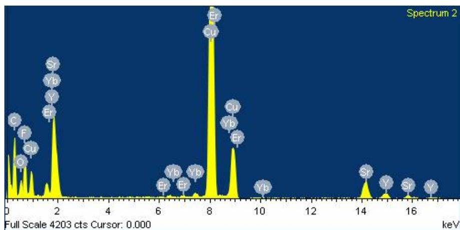
**Fig. S2** Energy dispersive X-ray (EDX) spectrum analysis of  $\text{Sr}_2\text{YF}_7:0.02\text{Er}^{3+}/0.18\text{Yb}^{3+}$  NPs ( $\sim 10$  nm), revealing the successful doping of  $\text{Er}^{3+}/\text{Yb}^{3+}$  into  $\text{Sr}_2\text{YF}_7$  host.
