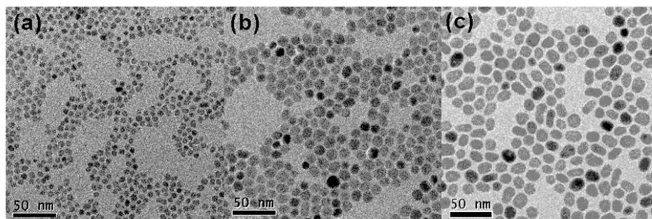
**Fig. S1** Transmission electron microscopy images of  $\text{Sr}_2\text{YF}_7:\text{Er}^{3+}/\text{Yb}^{3+}$  core-only nanoparticles (NPs) with different sizes: (a)  $6.1\pm 0.3$  nm, (b)  $10.7\pm 0.8$  nm and (c)  $12.9\pm 1.1$  nm, which were synthesized when the OA/ODE ratio (v/v) in the reaction solution was 10/7, 9/9 and 7/5, respectively.
