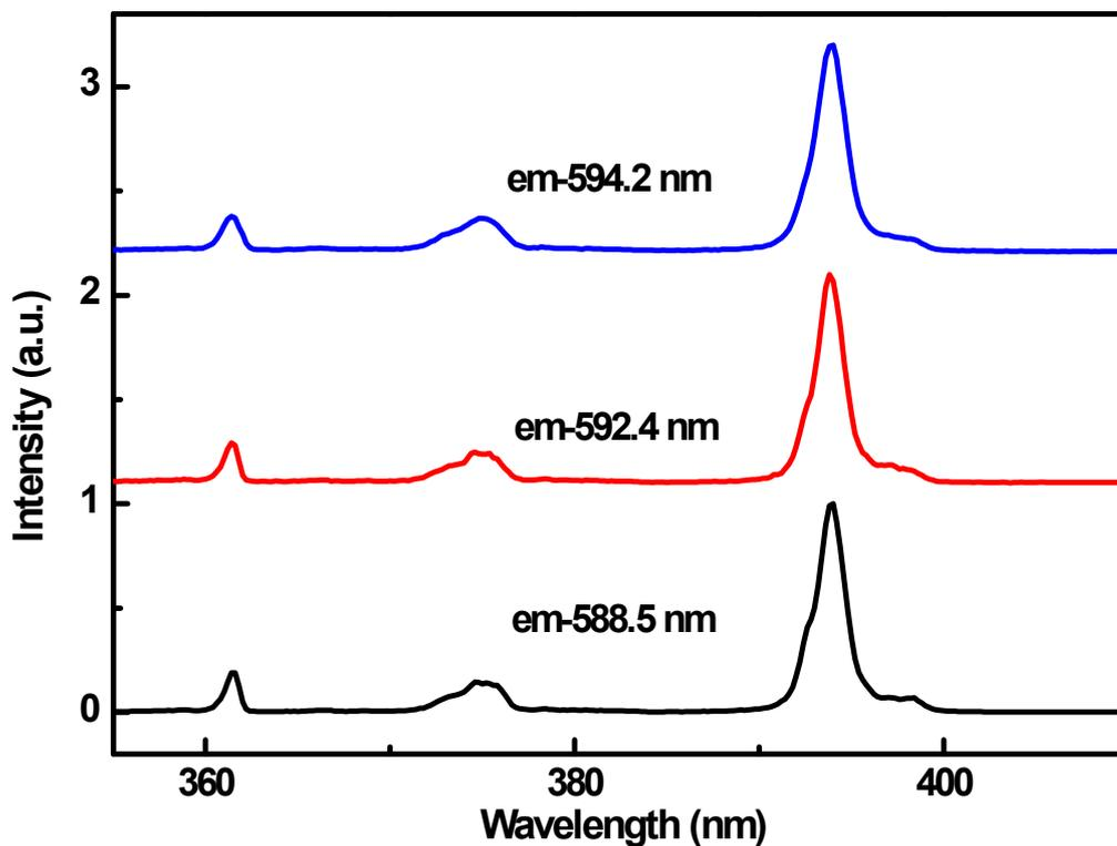
**Fig. S6** The 10-K photoluminescence (PL) excitation spectra of  ${}^5D_0 \rightarrow {}^7F_1$  of  $\text{Eu}^{3+}$  in  $\text{Sr}_2\text{YF}_7$  NPs by monitoring the emissions at 588.5, 592.4 and 594.2 nm, respectively. The line positions in these excitation spectra were observed to be identical, which indicates that these luminescent peaks originated from  $\text{Eu}^{3+}$  occupying the same spectroscopic site.
