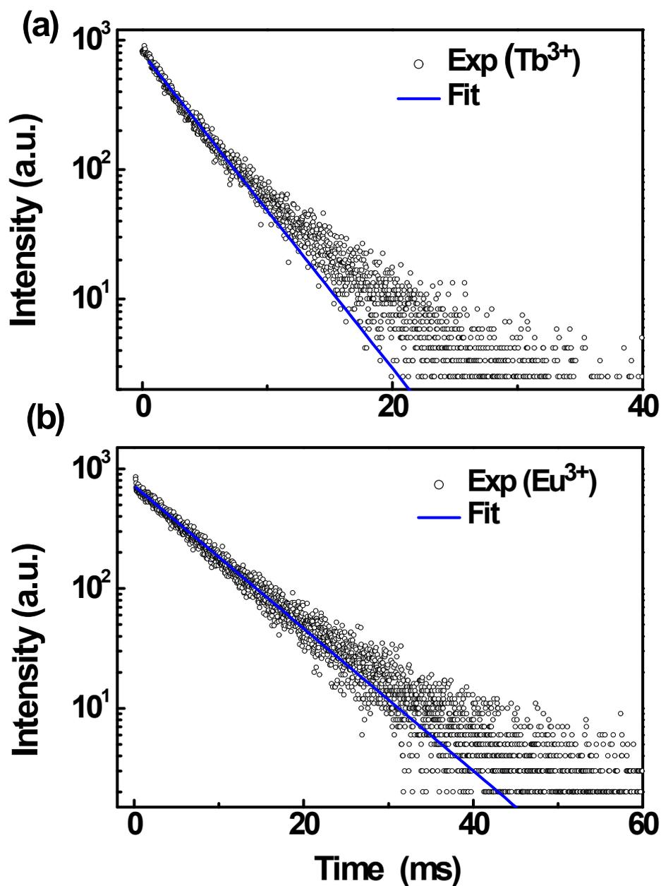
**Fig. S8** PL decays from (a)  $^5D_4$  of  $Tb^{3+}$  and (b)  $^5D_0$  of  $Eu^{3+}$  in  $Sr_2YF_7$  NPs at room temperature. Both decays were well fitted with single exponential function. The corresponding PL lifetimes were determined to be 3.7 ( $Tb^{3+}$ ) and 8.1 ( $Eu^{3+}$ ) ms, respectively.
