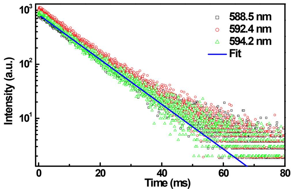
**Fig. S7** PL decays from  ${}^5D_0$  of  $\text{Eu}^{3+}$  in  $\text{Sr}_2\text{YF}_7$  NPs by monitoring the emissions at 588.5, 592.4 and 594.2 nm at 10 K. The PL lifetimes in all these decays were determined to be 10.5 ms by fitting with single exponential function.
