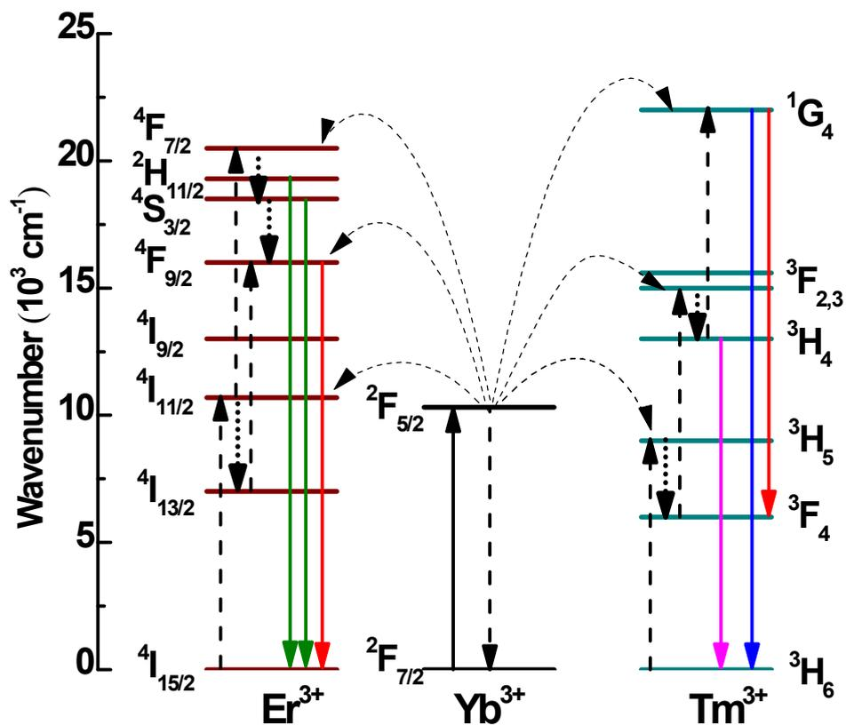
**Fig. S5** Schematic energy level diagrams showing typical UC processes for (a)  $\text{Er}^{3+}$  and (b)  $\text{Tm}^{3+}$  via the sensitization of  $\text{Yb}^{3+}$ . The dashed, dotted and full arrows represent the excitation, nonradiative relaxation, and emission processes, respectively.
