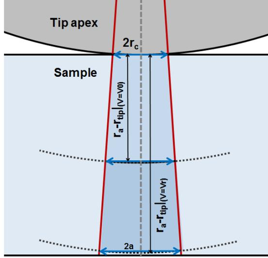
$R_S = 4.68 \text{ G}\Omega$  as experimentally determined with  $\rho_{\text{film}} = 4600 \text{ }\Omega\cdot\text{cm}$ ,  $a = 2.46 \text{ nm}$
