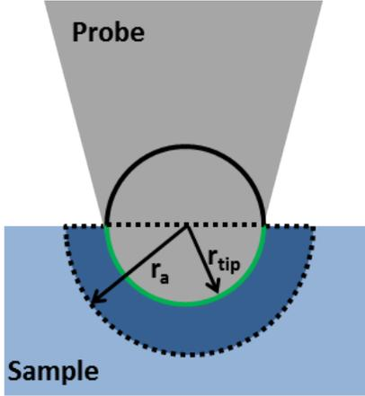
$r_c$  is the radius of the equivalent half buried sphere at the tip-sample contact and  $r_a$  is the radius of the hemisphere circumscribing the volume beneath the probe where charges accumulate
