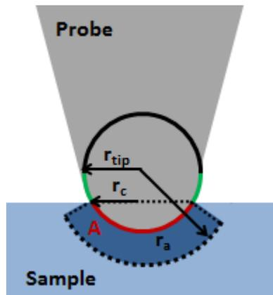
The area  $A$  of the cap sphere buried in the sample and in contact with the sample is given by
