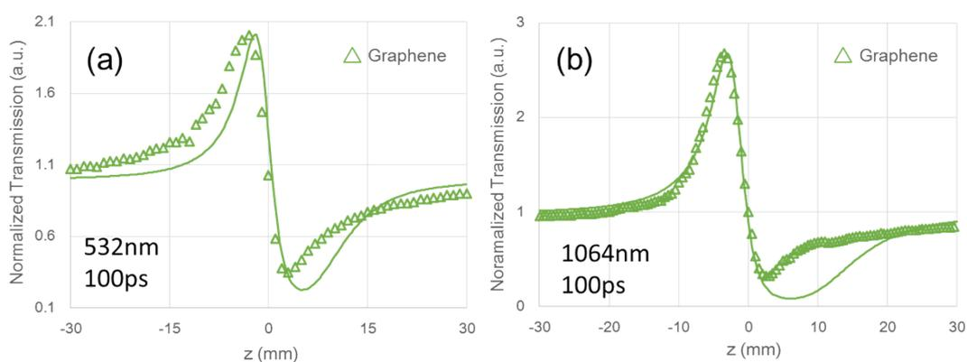
Figure S3 CA Z-scan results of graphene dispersions in ps region. Scatter trigons & solid lines denote for experimental results and theoretical fitting respectively.
