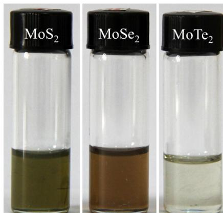
Figure S1 Photographs of  $\text{MoX}_2$  dispersions (3000 rpm) prepared by liquid phase exfoliation.
