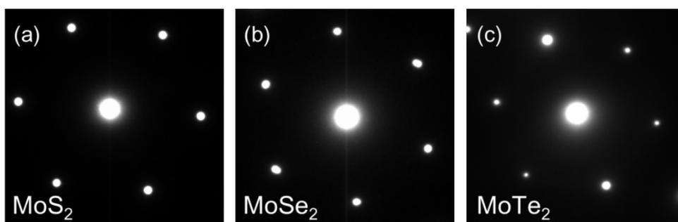
Figure S2 Electron scattering patterns from TEM characterizations of  $\text{MX}_2$  nanosheets.
