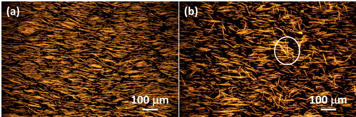
**Fig. S3.** Relatively high-density arrays obtained by two different methods. (a) Dense nanotube array compressed from a larger water surface area  $A_1$  to a smaller area  $A_2$  ( $A_1/A_2=1.7$ ). (b) Dense
