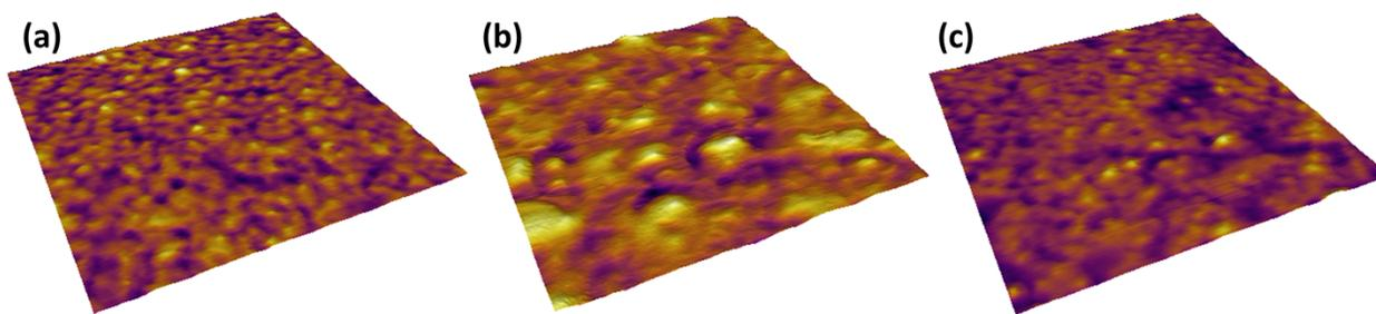
**Fig. S1.** Atomic Force Microscope images of the silicon surface. (a) The surface of a clean silicon substrate. (b) The surface of a silicon substrate contaminated with the surfactant. (c) The surface of a contaminated silicon substrate that was baked at 95°C for 15 min. The scan area is a 500 nm by 500 nm square.
