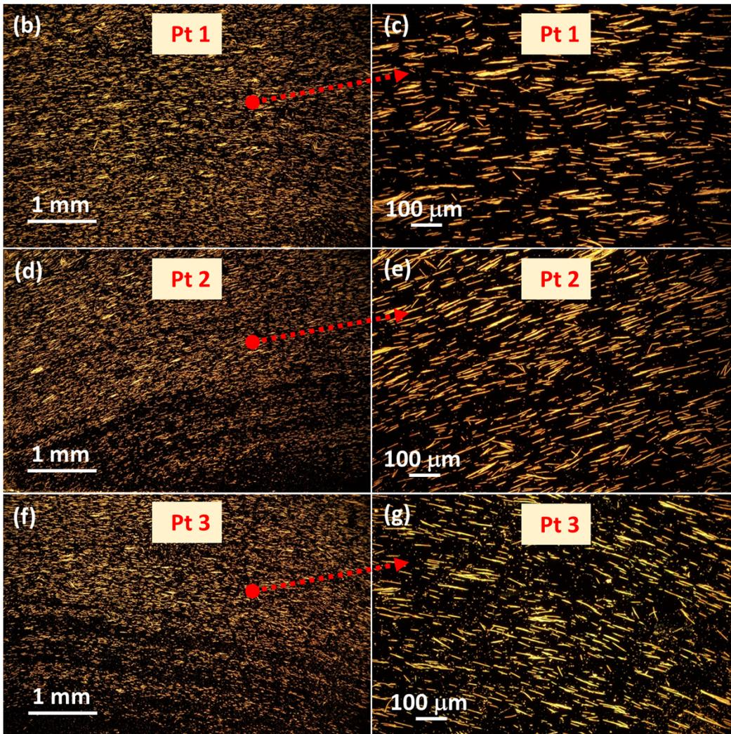
**Fig. S2.** The alignment of nanotubes on the water surface. (a) Schematic drawing showing the water surface and the receiving silicon substrates. The optical images of the aligned nanotubes at points Pt1, Pt2, and Pt3 are provided at lower magnifications in (b), (d), and (f), and higher magnifications in (c), (e), and (g), respectively. Note that (e) and (g) are from the dense area in (d) and (f).
