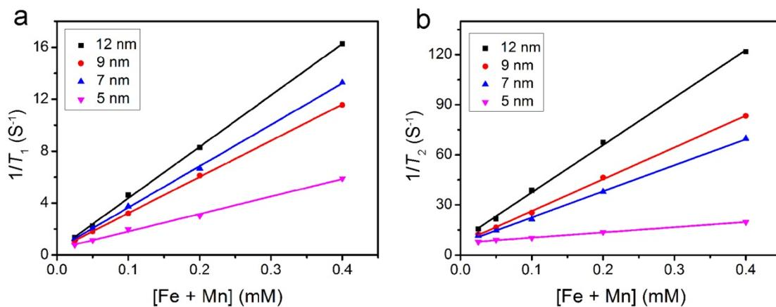
**Figure S5.** The linear fitting of (a) longitudinal and (b) transverse relaxation rates at 0.5 T versus magnetic metal (Fe + Mn) concentrations for 12 nm, 9 nm, 7 nm, and 5 nm MnIO nanoparticles.
