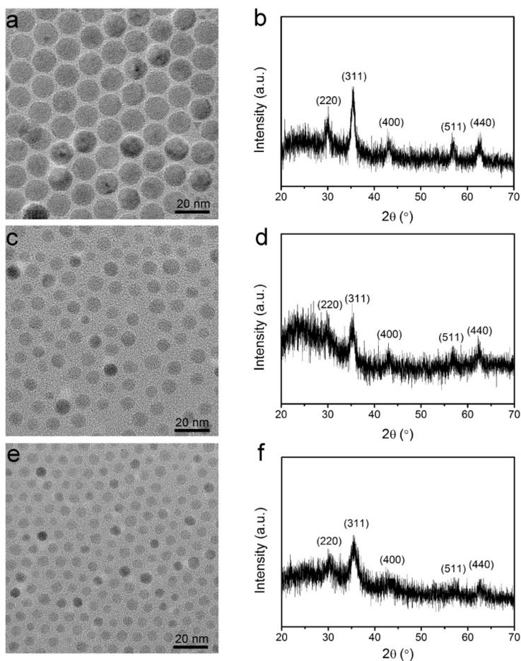
**Figure S6.** TEM images and XRD patterns of (a, b) 12 nm, (c, d) 7 nm, and (e, f) 5 nm IO nanoparticles, respectively.
