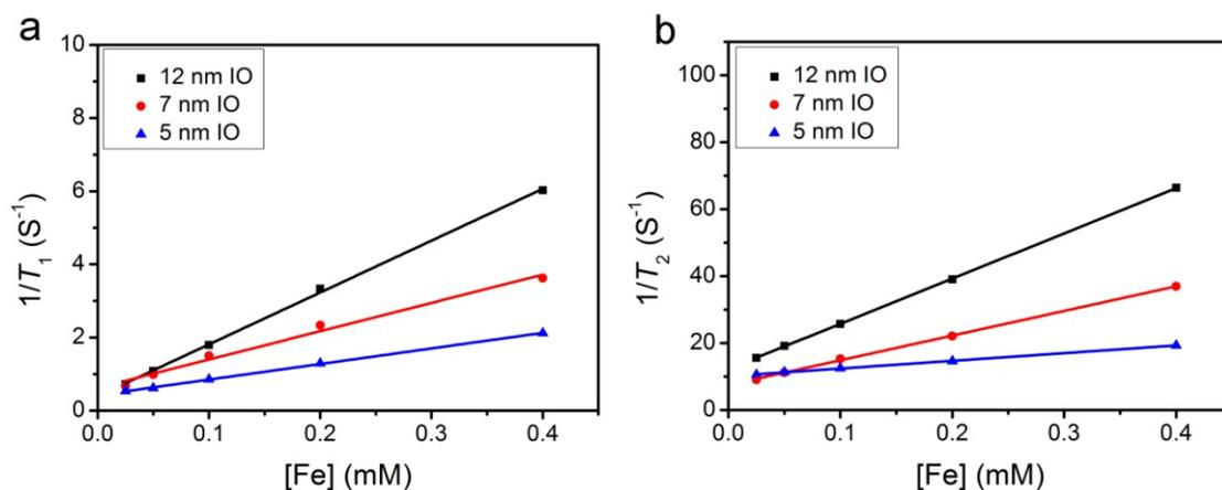
**Figure S7.** The linear fitting of (a) longitudinal and (b) transverse relaxation rates at 0.5 T versus Fe concentrations for 12 nm, 7 nm, and 5 nm IO nanoparticles.
