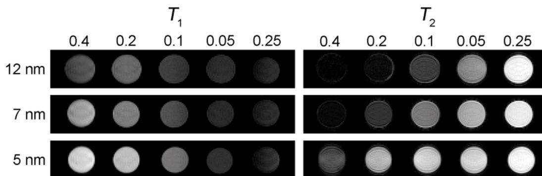
**Figure S10.**  $T_1$ - and  $T_2$ -weighted phantom images of 5 nm, 7 nm, and 12 nm MnIO nanoparticles in aqueous solution (containing 1% agar) with different metal ion (Fe + Mn, mM) concentrations at 7 T.
