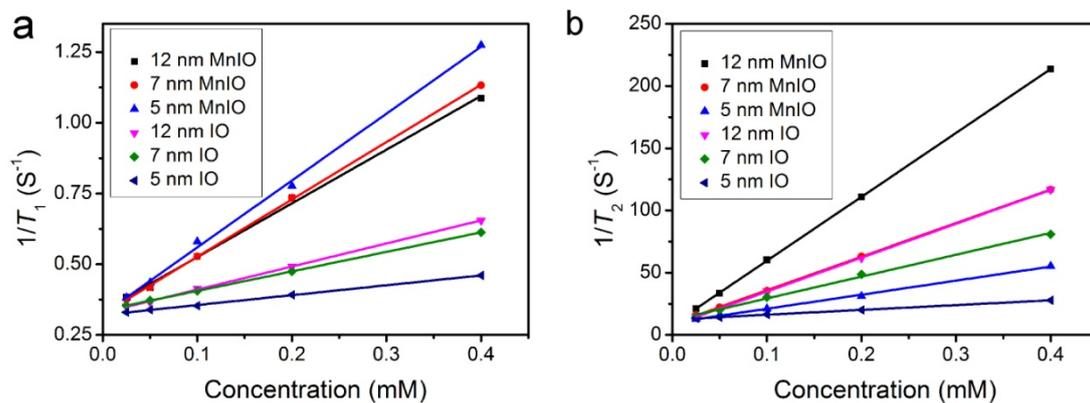
**Figure S9.** The linear fitting of (a) longitudinal and (b) transverse relaxation rates at 7 T versus metal ion ([Fe + Mn] for MnIO, [Fe] for IO) concentrations for 12 nm, 7 nm, and 5 nm MnIO or IO nanoparticles.
