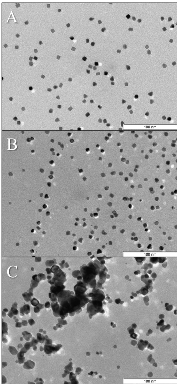
**Figure S2:** TEM images of Pt nanoparticles synthesized from  $\text{H}_2\text{PtCl}_6$  with a variety of silver salts at various concentrations as shape directing agents. The regularly shaped Pt nanoparticles in panels (A) and (B) support the hypothesis that silver can direct shape of platinum
