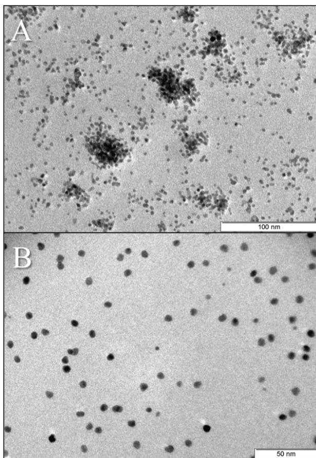
**Figure S4:** TEM images of Pt nanoparticles synthesized from  $\text{H}_2\text{PtCl}_6$  with copper salts as shape directing agents. The lack of significant particle shapes from either copper salt used at a broad range of concentrations (1%-200%) indicated that copper does not have similar shape directing properties to silver, despite some chemical similarities.  $\text{Cu}(\text{NO}_3)_2$  (A) and  $\text{CuBr}$  (B).
