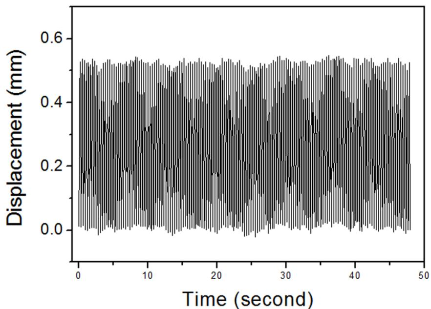
Fig. S4 Vibration displacement of the sG/PDMS bimorph under the 5Hz square wave voltage (0~10V).
