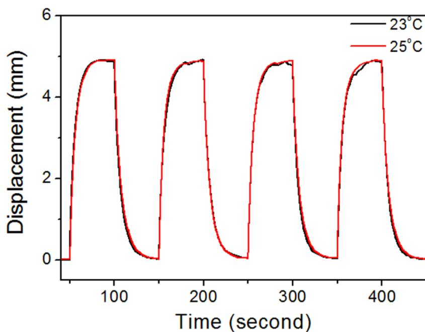
Fig. S1 0.01Hz square wave voltage (0~4V) actuated displacement of the sG/PDMS bimorph with different environmental temperature of 23°C and 25°C.
