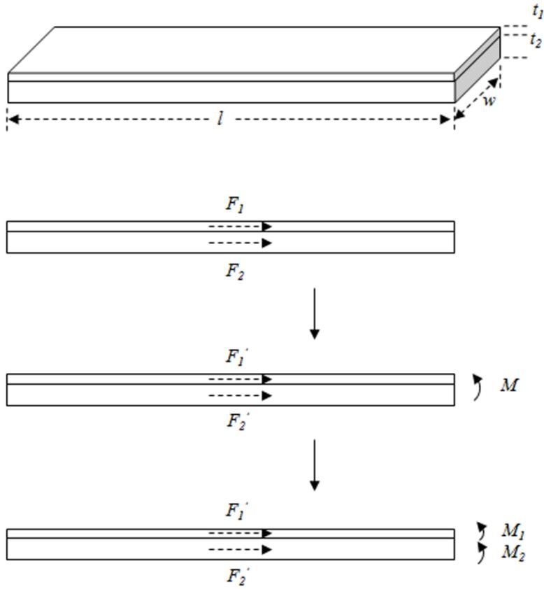
Fig. S3 Schematic diagram of force analysis of the thermal expansion induced bending deformation of the bimorph
