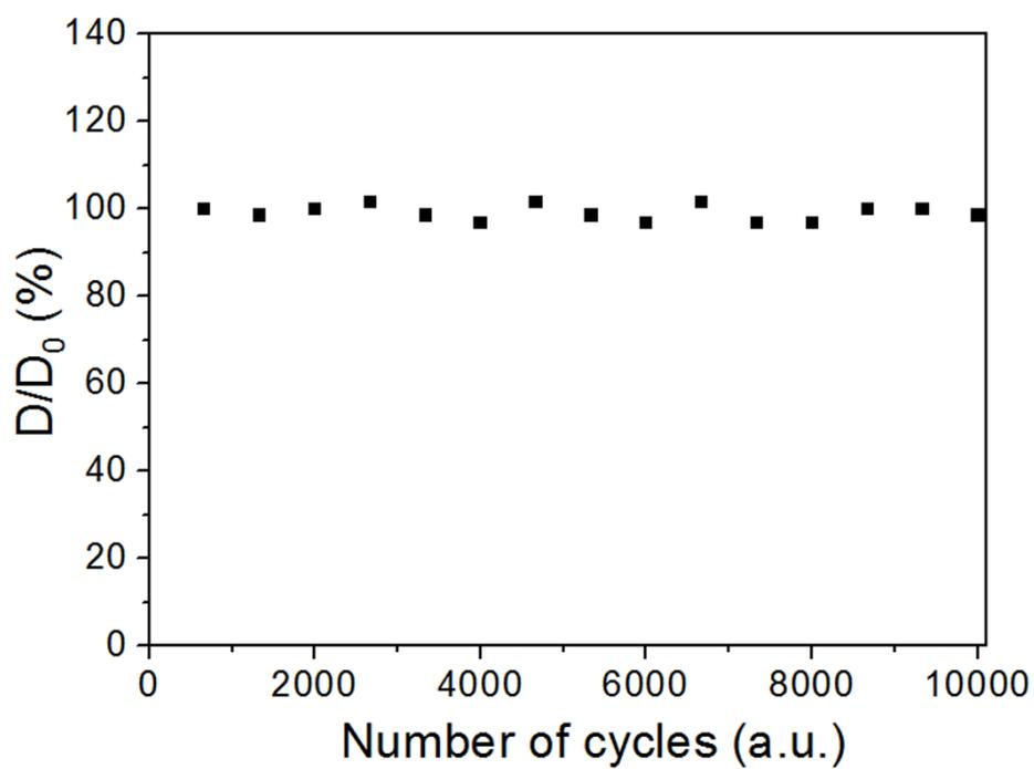
Fig. S5 Cycle life of the sG/PDMS bimorph with the 0.5Hz square wave voltage (0~5V) for about 10000 cycles.  $D_0$  represents the initial displacement value.
