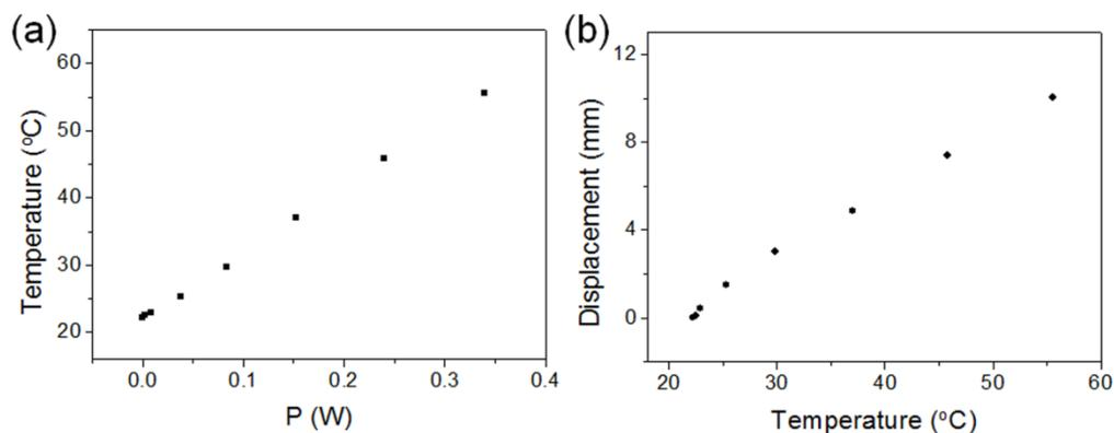
Fig. S2 (a) Generated temperature of the bimorph actuator versus the input electric power. (b) Maximum displacement of the bimorph actuator versus the generated temperature.
