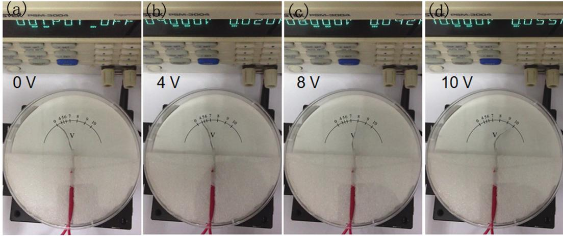
Fig. S6 A prototype voltmeter based on sG/PDMS bimorph actuator can measure the voltage ranging from 0V to 10V: (a) 0V, (b) 4V, (c) 8V, (d) 10V. The upper part of the images is a power supply, and the green numbers on its screen display corresponding output voltage.
