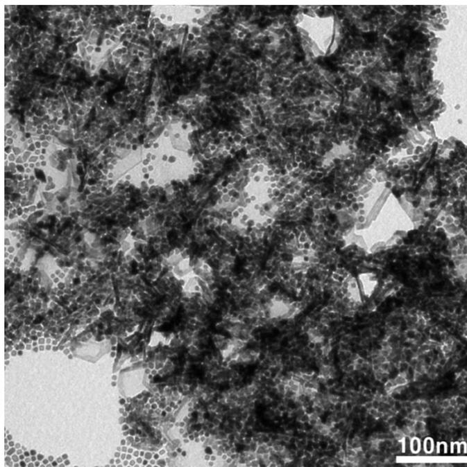
**Fig. S7** TEM images of Pt/Pd ratio dependent structural evolution of PdPt nanostructures. The amount of formed PdPt nanosheet decreases as Pt/Pd ratio increases.
