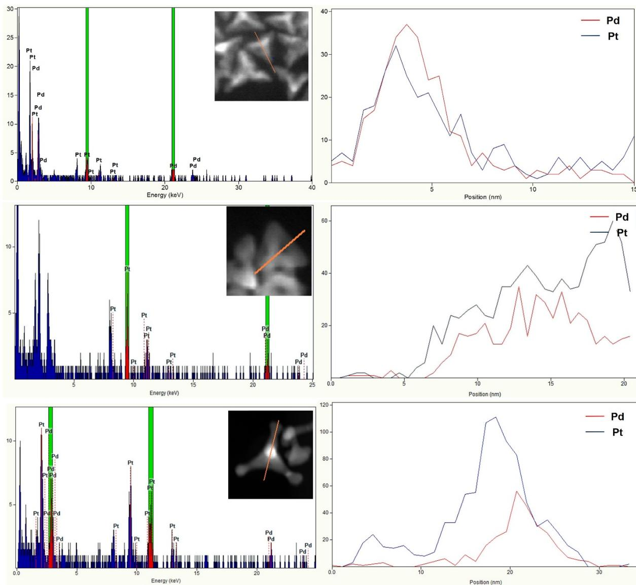
**Fig. S4** Energy dispersive X-ray spectrum of a PdPt alloy nanotent structure, Pt popped out PdPt nanostructure, and Pt overgrown PdPt nanostructure.
