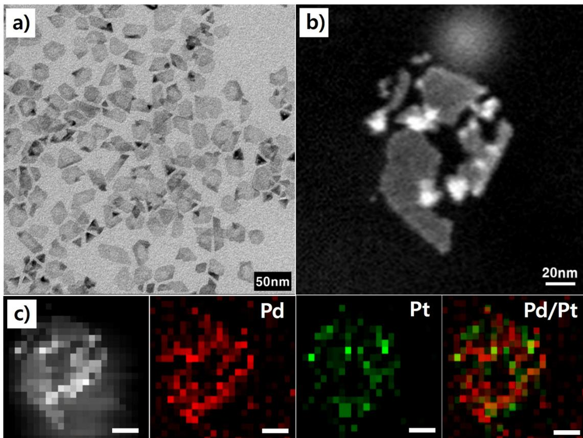
**Fig. S6** TEM image of products from thermal decomposition of  $\text{Pt}(\text{acac})_2$  and  $\text{Pd}(\text{acac})_2$  at high temperature of 200 °C under CO. Separate formation of Pd nanosheet and Pt nanocube is obvious.
