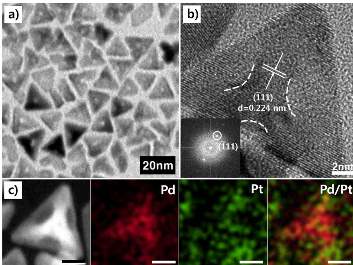
**Fig. S9** HRTEM images of a PdPt nanotent structure completely filled with Pt, which is found as a minor product from a reaction described in Fig. 3a.
