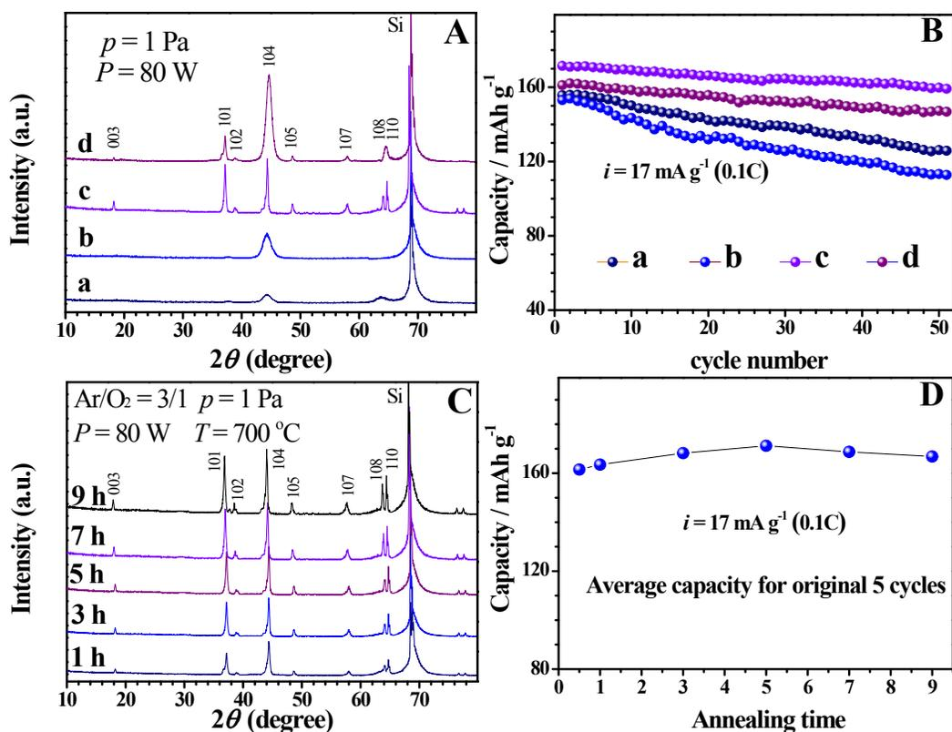
**Figure 2S** (A) XRD patterns and (B) Cycle performance of thin films, which are deposited in Ar/O<sub>2</sub> (3:1) at (a) room temperature, (c) annealed at 700 °C, and deposited in pure Ar at (b) room temperature and (d) annealed at 700 °C; (C) XRD patterns and (D) discharge capacity versus annealing time of 700 °C annealed films. Cycling curves (B, D) are recorded using coin-type half-cell between 2.8 and 4.5 V at a current density of 17 mA g<sup>-1</sup>.
