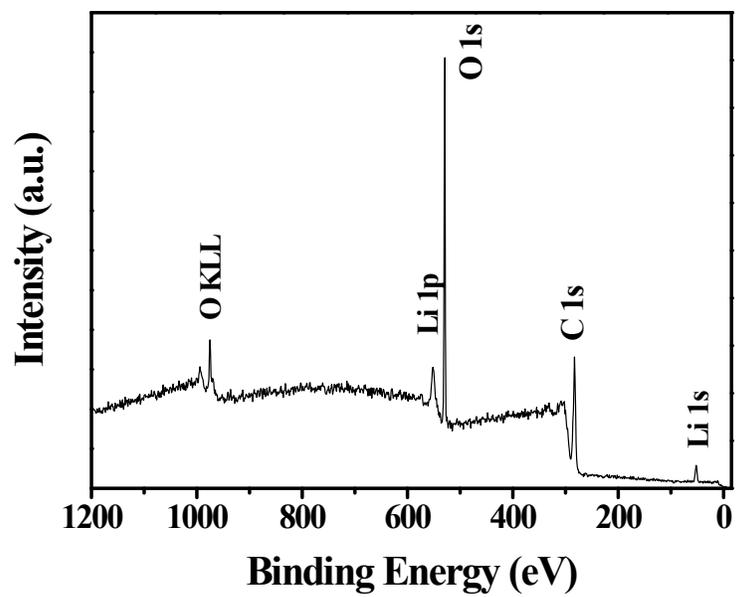
**Figure 1S** XPS survey spectrum of the as-deposited Li-Co-Ni-Mn oxide thin film.
