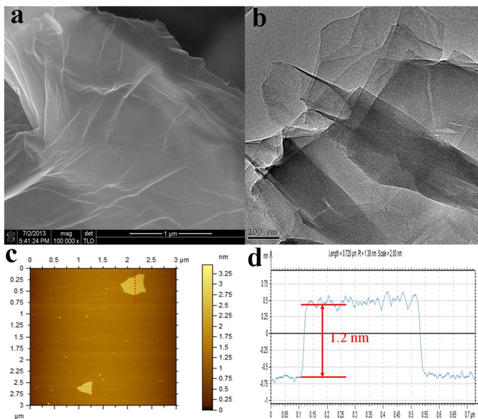
**Figure S1.** (a) FESEM, (b) TEM, (c) AFM image and (d) corresponding height profile of GO aqueous solution.
