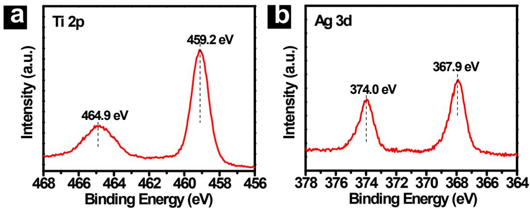
**Figure S7.** High-resolution XPS spectra of Ag 3d and Ti 2p of Ag/GR/SC-TNBs ternary heterostructure after recycling photocatalytic reactions.
