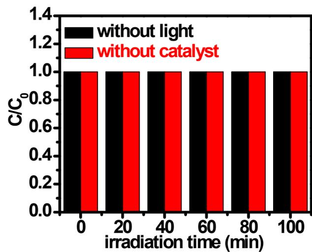
**Figure S5.** Blank experiments for photodegradation of RhB without light and catalyst.
