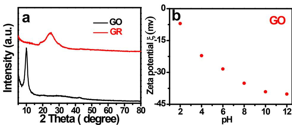
**Figure S2.** (a) XRD patterns of GO and GR, and (b) Zeta potential of GO aqueous solutions.
