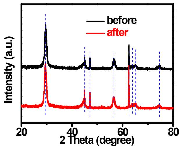
**Figure S6.** XRD patterns of Ag/GR/SC-TNBs ternary heterostructure before and after recycling photocatalytic reactions.
