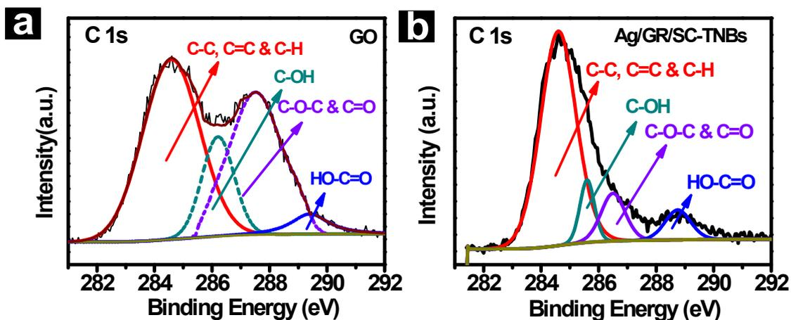
**Figure S3.** High-resolution XPS spectra of C 1s for (a) GO and (b) Ag/GR/SC-TNBs ternary heterostructure.
