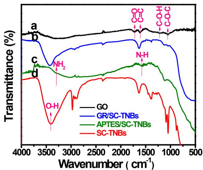
**Figure S4.** FTIR spectra of (a) GO, (b) GR/SC-TNBs, (c) APTES-SC-TNBs, and (d) SC-TNBs.
