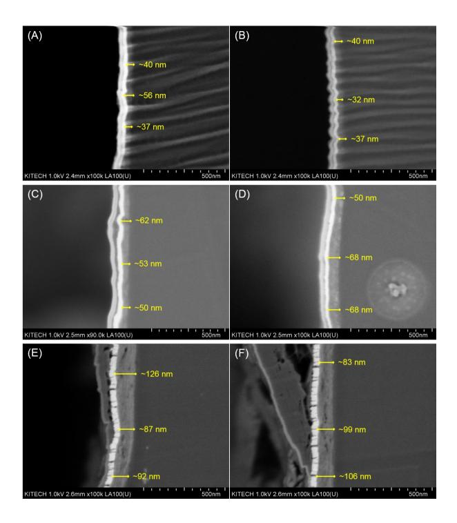
**Fig. S1** Cross-sectional SEM images of the (A and B) GO alone, (B and C)  $GO_{1.9}/LN_{0.1}$ , (C and D)  $GO_{1.5}/LN_{0.5}$ -coated PET films.
