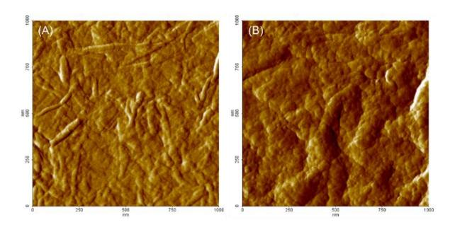
Fig. S2 AFM images of upper surfaces of the (A) GO alone and (B)  $GO_{1.9}/LN_{0.1}$ .
