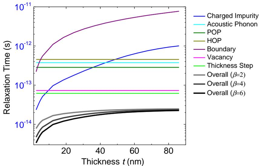
**Fig. S2:** Relaxation time for different scattering mechanisms with different MoS<sub>2</sub> thickness.
