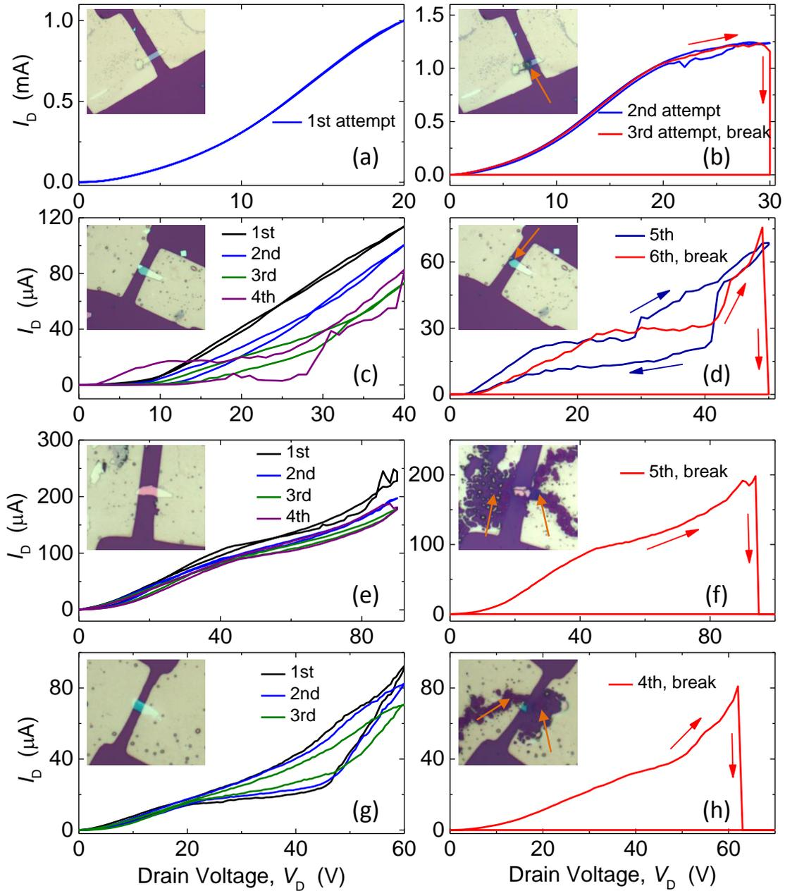
**Fig. S1:**  $V_D$  sweeps during the electrical breakdown measurement of multilayer MoS<sub>2</sub> transistors shown in Fig. 4 in the main text, with (a)-(b) for the device in Fig. 4(a), (c)-(d) for the device in Fig. 4(b), (e)-(f) for the device in Fig. 4(c), and (g)-(h) for the device in Fig. 4(d). The red curves show the final breakdown sweeps. Insets: Optical microscope images before (a,c,e,g) and after (b,d,f,h) the breakdown.
