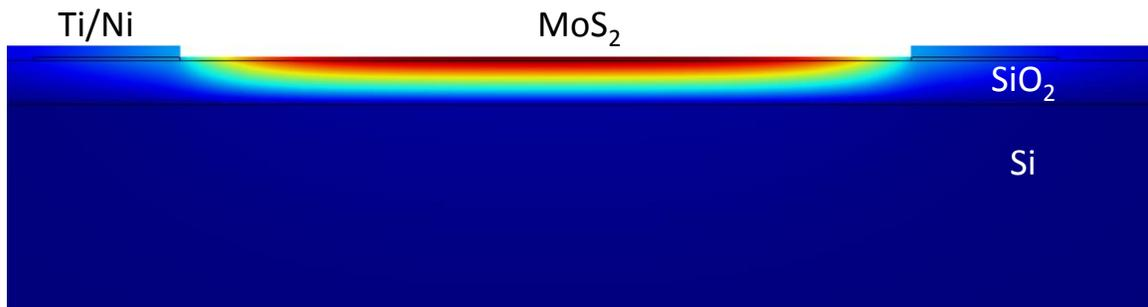
**Fig. S3:** The cross-section view of the FEM result of the temperature profile under Joule heating. In simulation the  $\text{MoS}_2$  has  $t=25\text{nm}$ ,  $L=5\mu\text{m}$ ,  $W=2\mu\text{m}$ .
