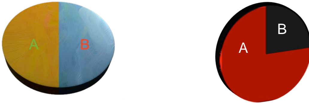
Figure 1. Showing the different types of section target arrangement used for the production of nanoparticles.
