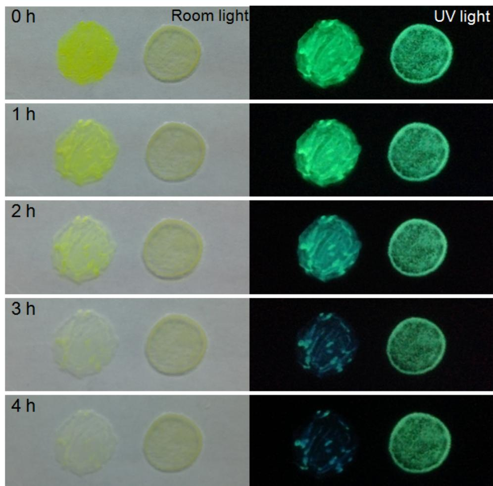
**Fig. S5** Optical images of the commercial fluorescent dye ink (the first and third columns) and starch/g-CD phosphors (mass ratio 45:1) (the second and fourth columns) deposited on glass substrates exposed under 500 W xenon-mercury lamp for different time.
