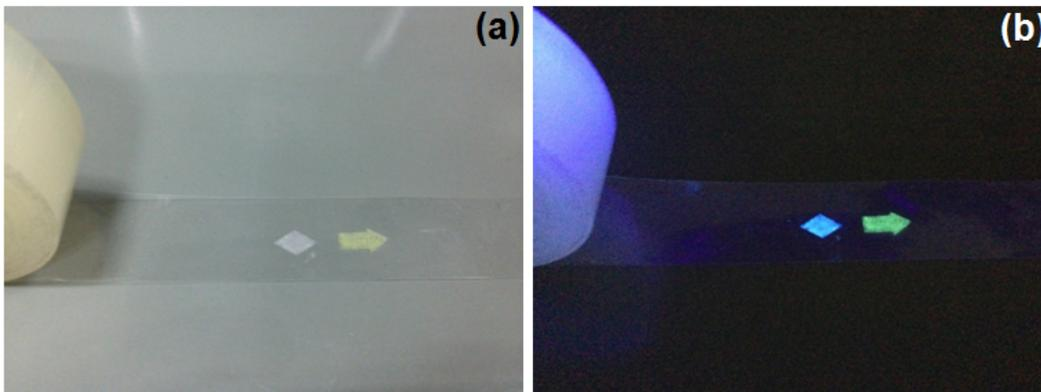
**Fig. S6** Optical images of the patterns composed by blue or green luminescent phosphors in specific shapes on transparent tape under room light (a) and UV excitation (b).
