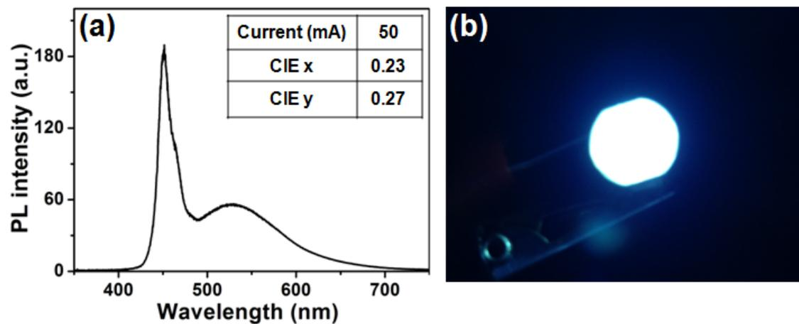
**Fig. S4** (a) Emission spectrum of the starch/g-CD phosphor-based (mass ratio: 70:1) LEDs. (b) Optical image of the corresponding LEDs at the current of 50 mA.
