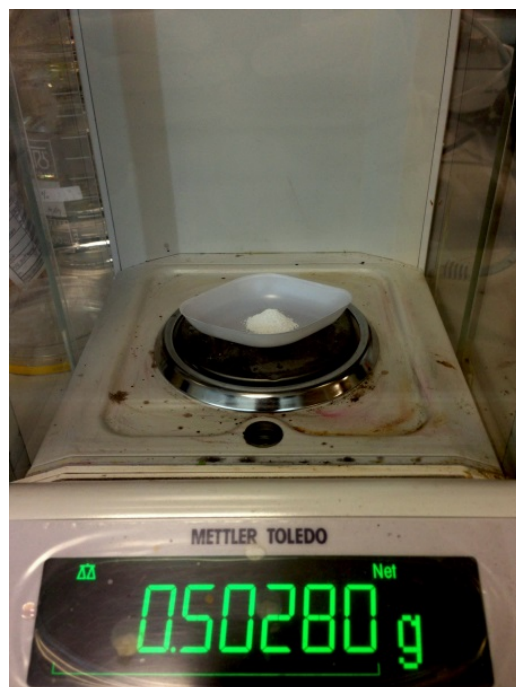
Fig. S4 Digital photograph of TiO 2 microspheres synthesized from one-pot synthesis. In one typical synthesis process, 2 ml of titanium isopropoxide could produce 502.8 mg of TiO 2 microspheres (after calcination at 400 °C for 2 hours), and the product yield is as high as ~ 96.1%.
