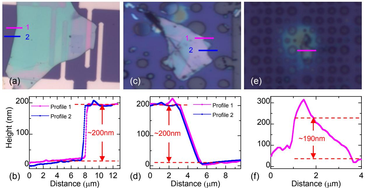
**Figure S3:** Device thickness measurement with AFM. (a,c,e) Optical microscope images of the devices. (b,d,f) Height measurement of the solid lines indicated in (a), (c), and (e), respectively. (a,b) show the same device in Fig. 1 of Main Text, (c,d) show the device in Fig. 4b and 4d of Main Text, and (e,f) show the device in Fig. 4c of Main Text.
