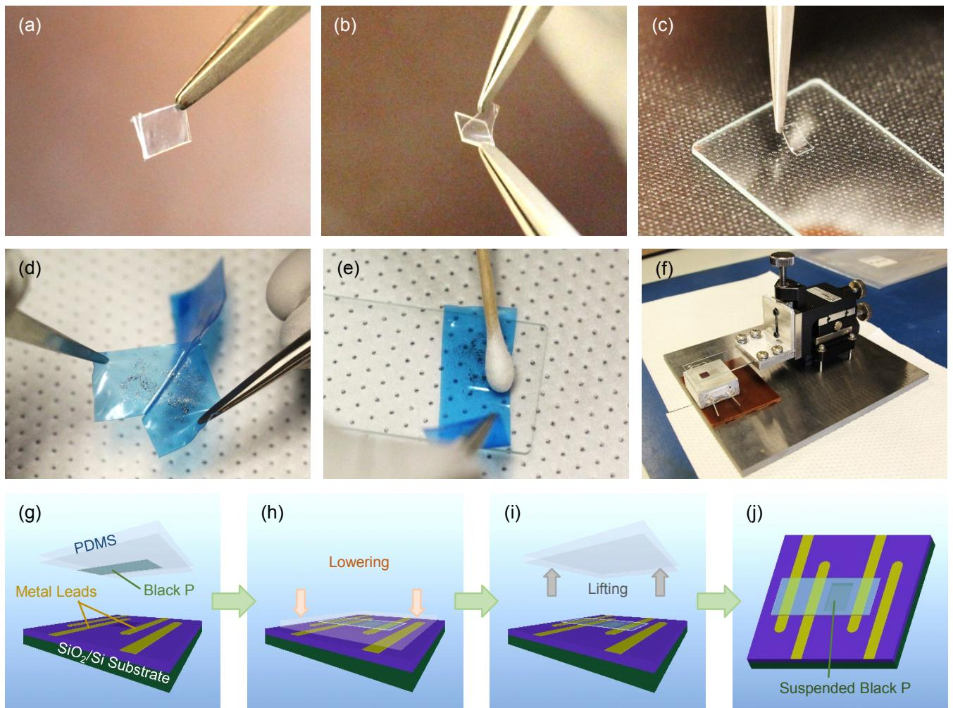
**Figure S1:** Fabrication process of suspended black P nanoelectromechanical resonators. (a-f) Images of black P flakes exfoliation and transfer preparation steps. (g-j) Schematic of the transfer process. (g) Aligning the black P flake on PDMS to the prefabricated substrate patterns. (h) Lowering the PDMS stamp to bring the black P flake and substrate into contact. (i) Lifting up the PDMS stamp with the black P flake remaining on the substrate. (j) The resulting device.
