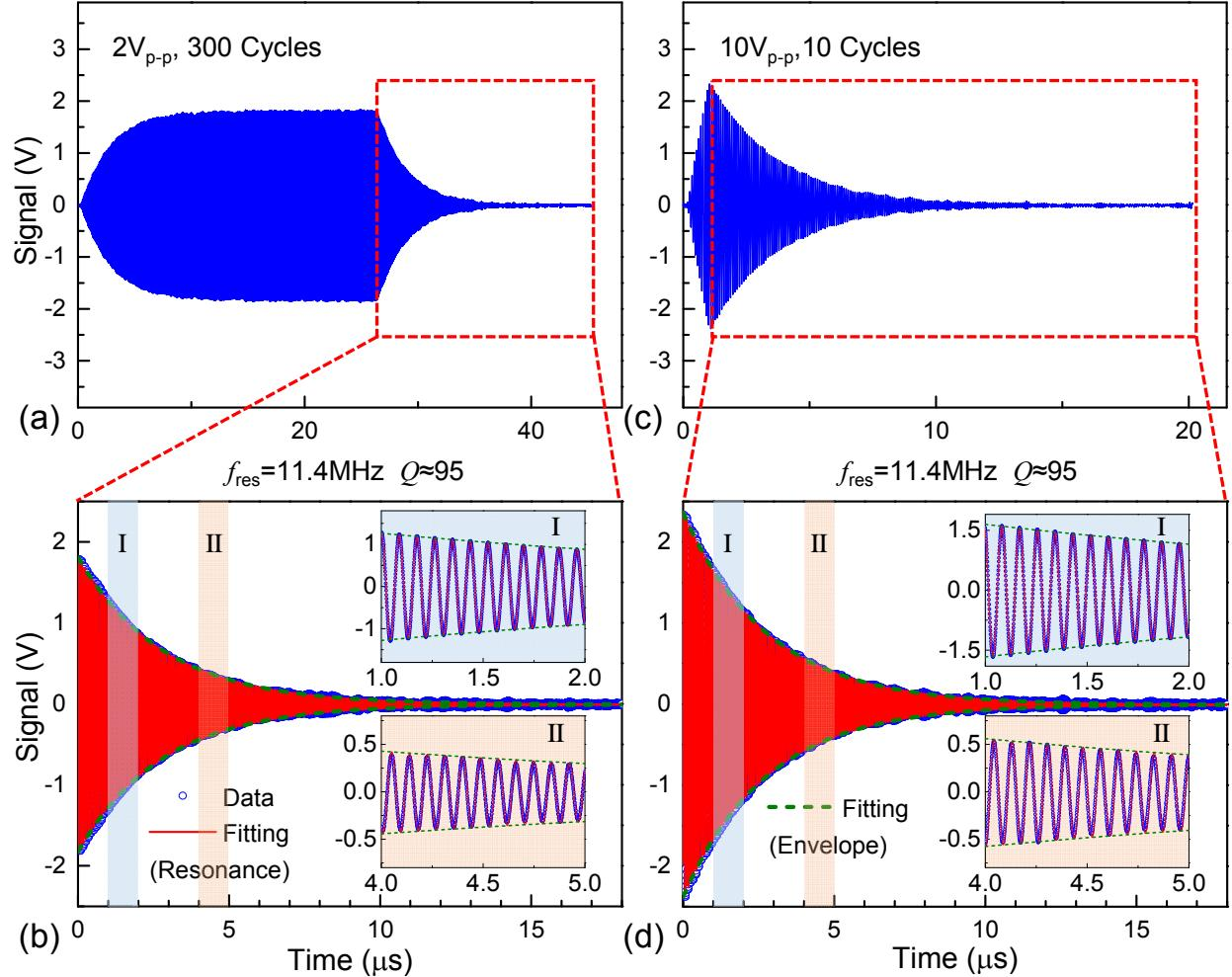
**Figure S2:** Fitting to the time-domain ring-down measurement. (a) Ring-down data for a 300 cycle burst with amplitude of  $2V_{p-p}$ . (b) Fitting to the ring-down data in (a) shown by the red dashed box. (c) Ring-down data for a 10 cycle burst with amplitude of  $10V_{p-p}$ . (d) Fitting to the ring-down data in (c) shown by the red dashed box. Insets in (b) and (d) show the zoom-in views of the fitting in the corresponding regions (I and II) as shown by the shaded area in (b) and (d).
