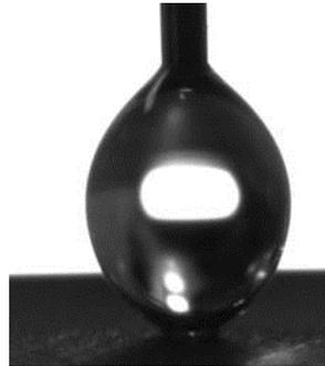
**Figure S4.** A photograph of shape deformation on rough SS before detachment, leading to the calculated adhesion force between the water droplet and Ni(OH)<sub>2</sub>/SS of 33μN by balancing vertical forces, as shown in equation (S1)
