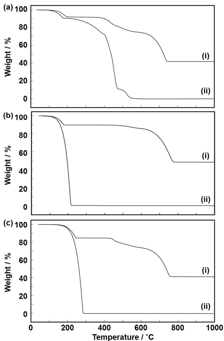
**Fig. S1.** TG curves of the composites based on VCz (a), AB (b), and PY (c). The spectra (i) and (ii) correspond to the composites and the commercial organic crystals respectively.
