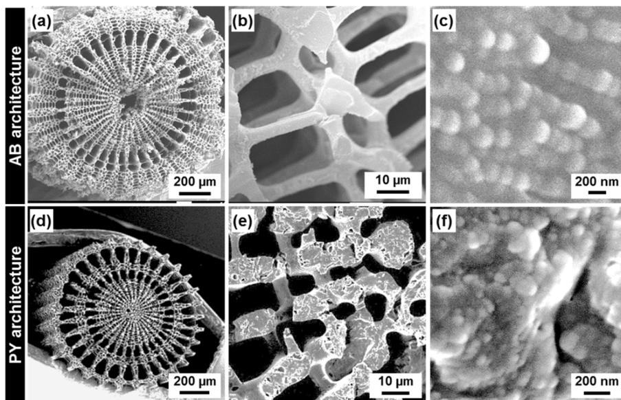
**Fig. S2.** FESEM images of the replicated architectures of AB (a–c) and PY (d–f) crystals.
