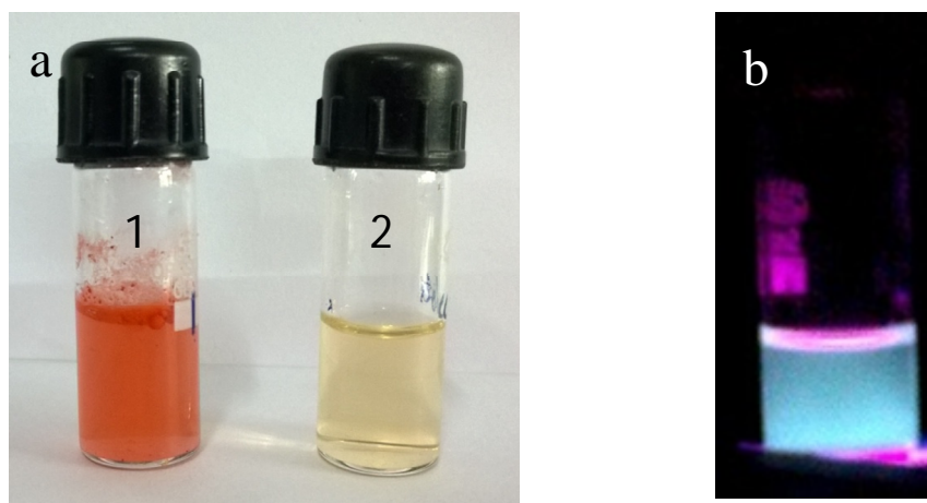
Figure S1. Digital images of (a) \beta -carotene dispersed in water (1) and after formation of C-dots (2). (b) C-dot solution showing blue fluorescence under UV light ( \lambda_{\text{ex}} = 365 nm).
