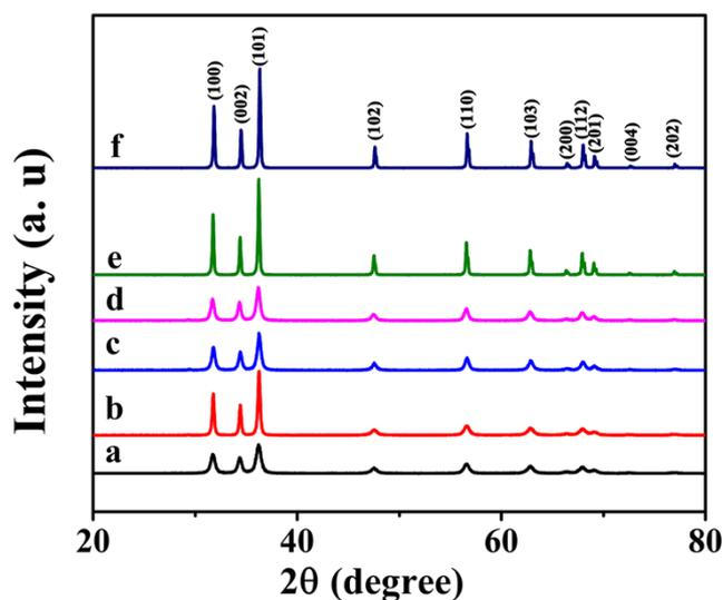
Fig. S1 XRD of ZnO NPs. (a) ZnO-1; (b) ZnO-2; (c) ZnO-3; (d) ZnO-4; (e) ZnO-5; (f) ZnO-6. All diffraction peaks can be perfectly
