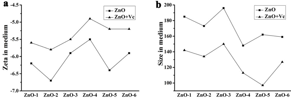
Fig. S5 Zeta potential and size of ZnO NPs with or without Vc in medium. (a) Zeta potential; (b) size.
