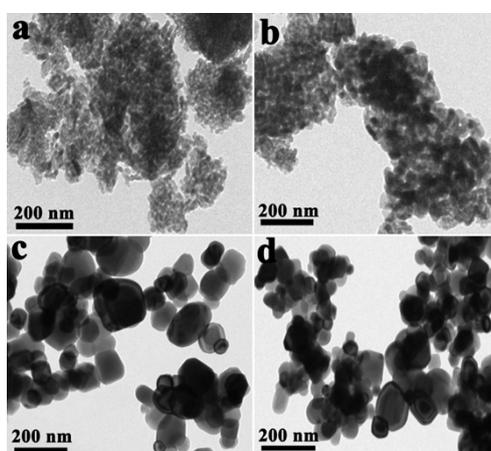
Fig. S6 TEM images of TiO<sub>2</sub> NPs. (a) TiO<sub>2</sub>-1; (b) TiO<sub>2</sub>-2; (c) TiO<sub>2</sub>-3; (d) TiO<sub>2</sub>-4.
