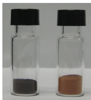
Fig. S3 Photographs of PDA@Fe 3 O 4 @SiO 2 (left) and the derivative Fe 2 O 3 @SiO 2 (right) composite spheres after calcination at 600 °C in air.
