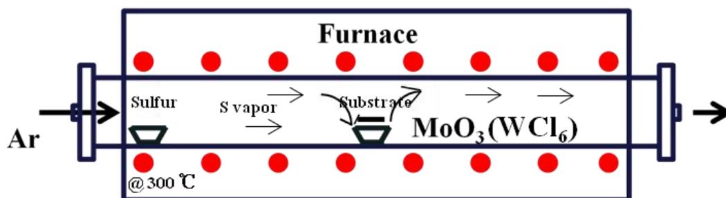
**Fig. S1** Schematic diagram of the reaction setup used for growing the atomically thin MoS<sub>2</sub> and WS<sub>2</sub> nanosheets by chemical vapor deposition.
