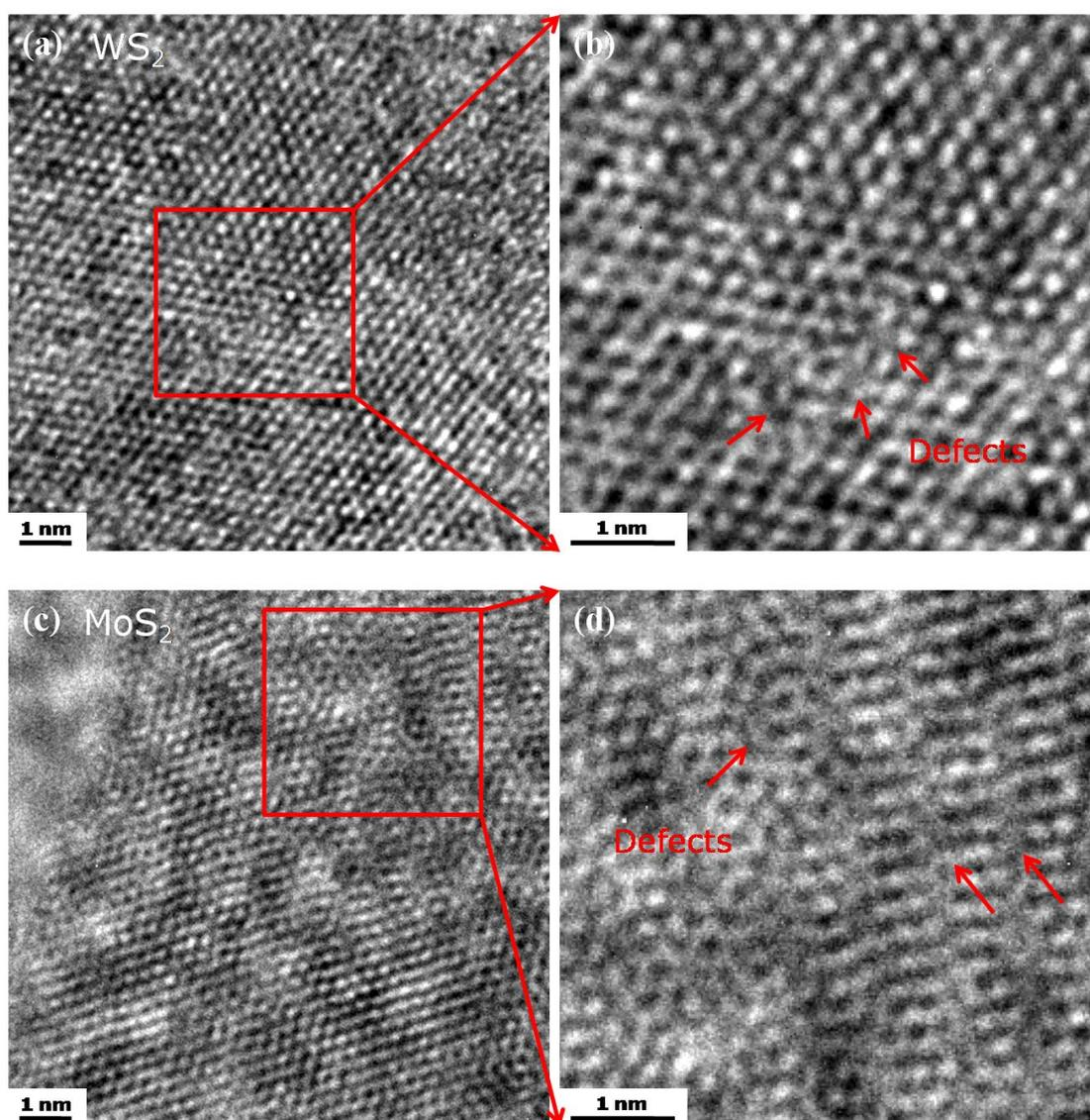
**Fig. S5** HRTEM images of WS<sub>2</sub> (a, b) and MoS<sub>2</sub> (c, d) nanosheets. The defects and dislocations exist clearly in both nanosheet systems.
