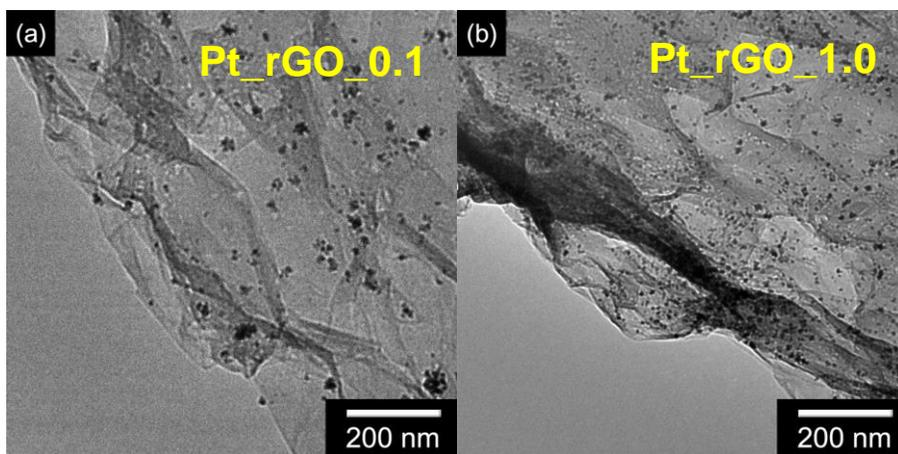
**Figure S1.** TEM images of (a) Pt\_rGO\_0.1 and (b) Pt\_rGO\_1.0 sheets.
