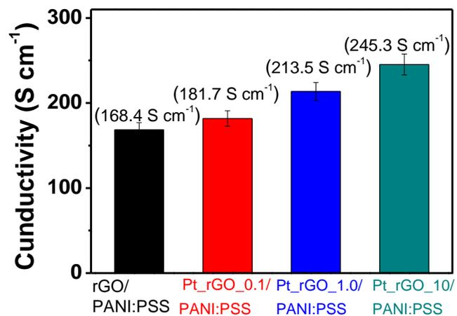
**Figure S3.** Electrical conductivity of Pt\_rGO/PANI:PSS with different Pt amount (black: Pt\_rGO\_0.1/PANI:PSS; red: Pt\_rGO\_1.0/PANI:PSS; blue: Pt\_rGO\_10/PANI:PSS).
