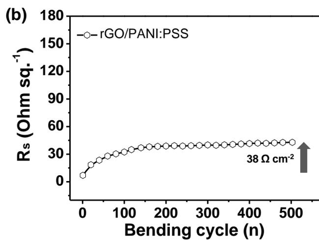
**Figure S4.** Surface resistance changes of (a) PANI:PSS and (b) rGO/PANI:PSS micropatterns with enhancing of bending cycles.
