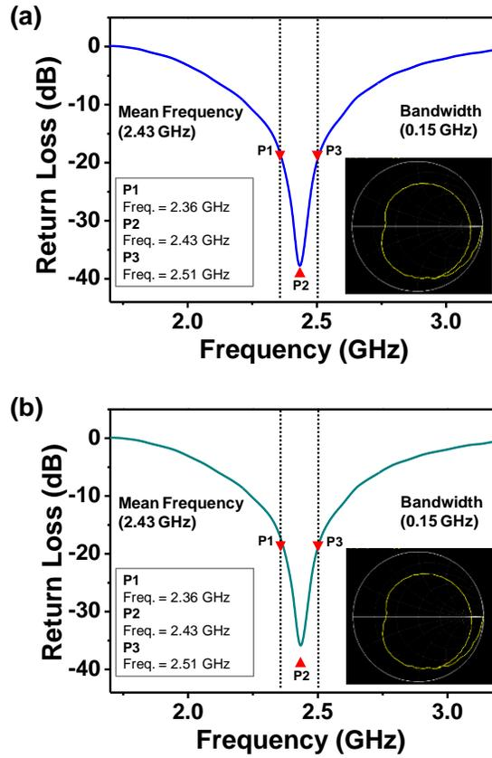
**Figure S5.** Return loss curve of the dipole tag antenna (a) under bending 90 degree and (b) after bending using Pt\_rGO/PANI:PSS-based electrode (inset: Smith chart impedance diagram).
