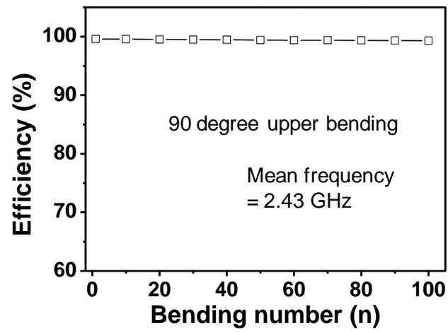
**Figure S6.** Transmitted power efficiency at mean frequency (2.43 GHz) with bending cycles.
