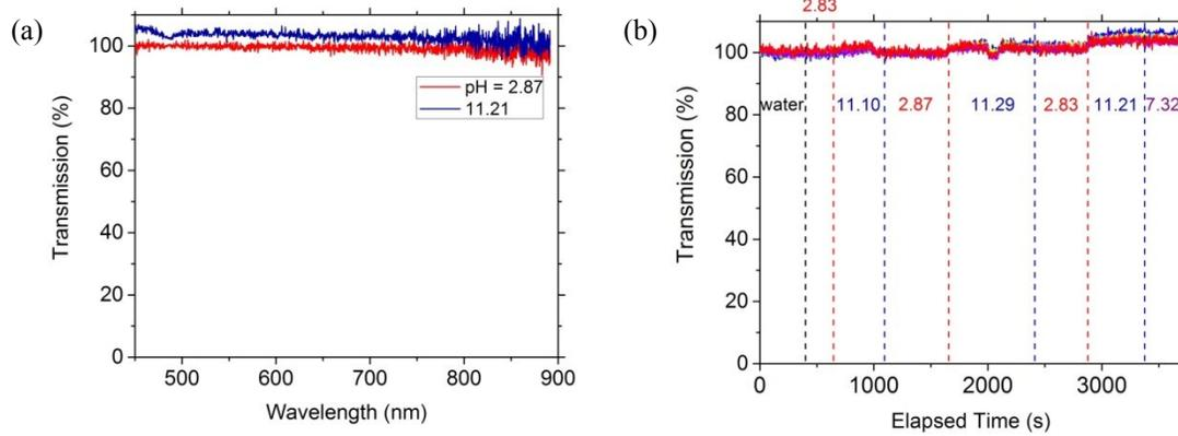
**Figure S10.** pH sensing using a Au nanoparticles coated optical fiber calcined at 200 °C using KOH and H<sub>2</sub>SO<sub>4</sub> acid/base pair. The transmission at the plasmon absorption peak 550 nm as a function of time when the pH of the solution is repeatedly adjusted by adding KOH/H<sub>2</sub>SO<sub>4</sub>. The pH of the solution is denoted by the numbers in the figure.
