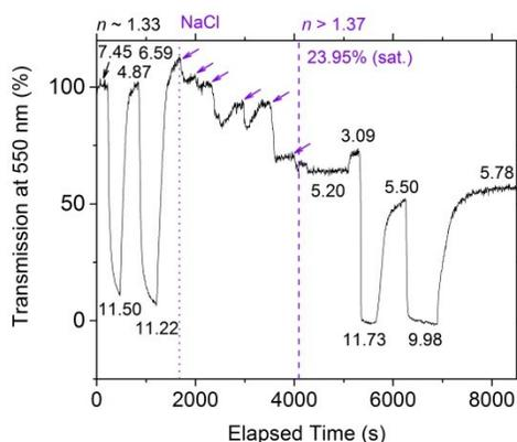
**Figure S12.** Transmission spectra of a Au coated optical fiber calcined at 200 °C in solution as different amounts of NaCl are added as indicated by the wt.% in the legend. A red-shift in the plasmon absorption band is clearly observed as the  $n$  increases, as expected, despite the fact that the change in transmission ( $\sim 35\%$ ) is much smaller compared to the change in response to pH ( $\sim 80\%$ ).
