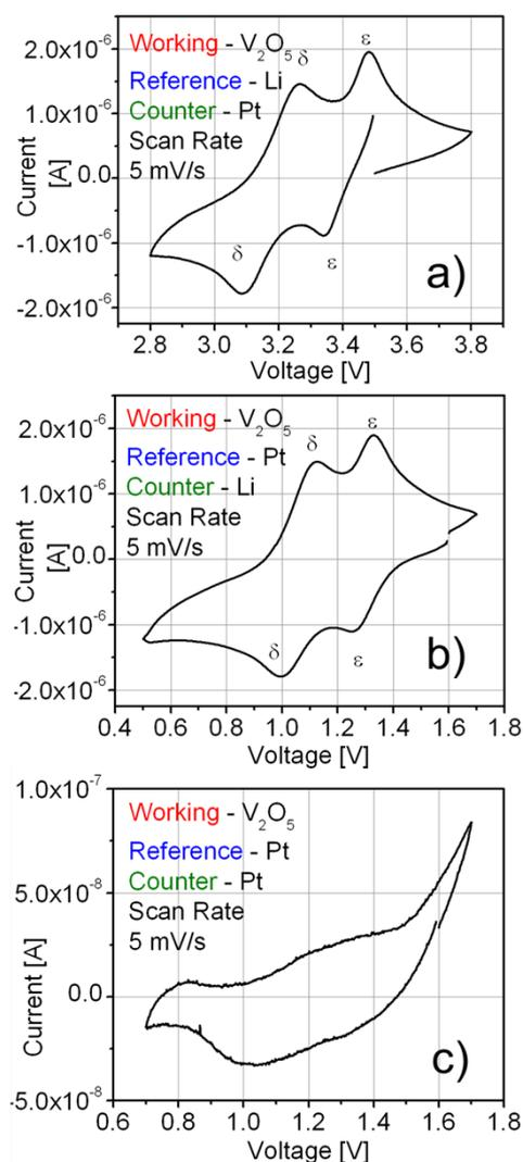
**Figure S2.** Multi-nanowire  $Pd/V_2O_5$  electrodes voltammograms measured with: a) RE – Li, CE – Pt; b) RE – Pt, CE – Li; c) RE – Pt, CE – Pt.
