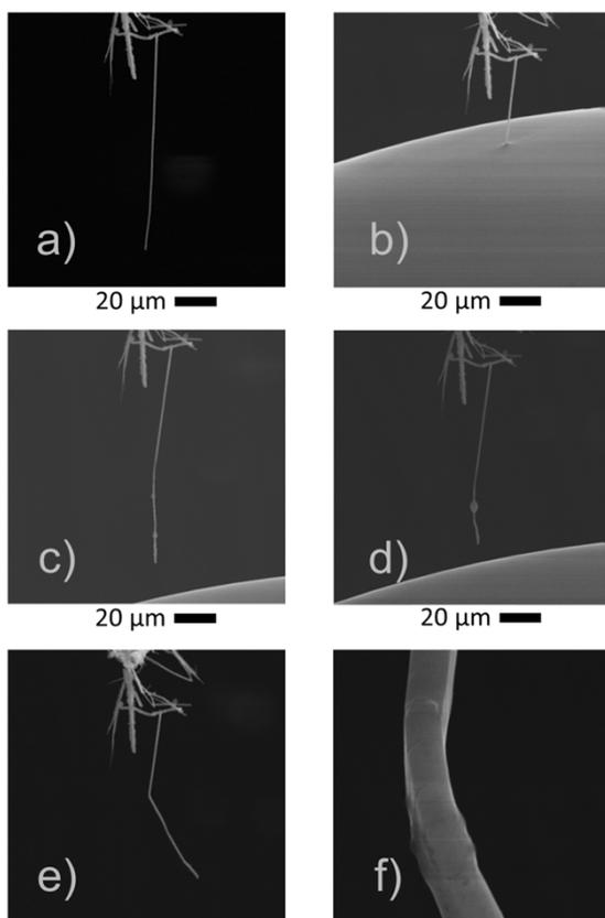
**Figure S1.** *In situ* morphological changes - bending: a) Initial shape of a  $V_2O_5$  whisker; b) Whisker submerged into electrolyte; c) Whisker pulled out of electrolyte after 2 charge-discharge cycles; d) after 3 cycles; e) final whisker distortion after 5 cycles; f) zoomed-in image of the formed kink in e).
