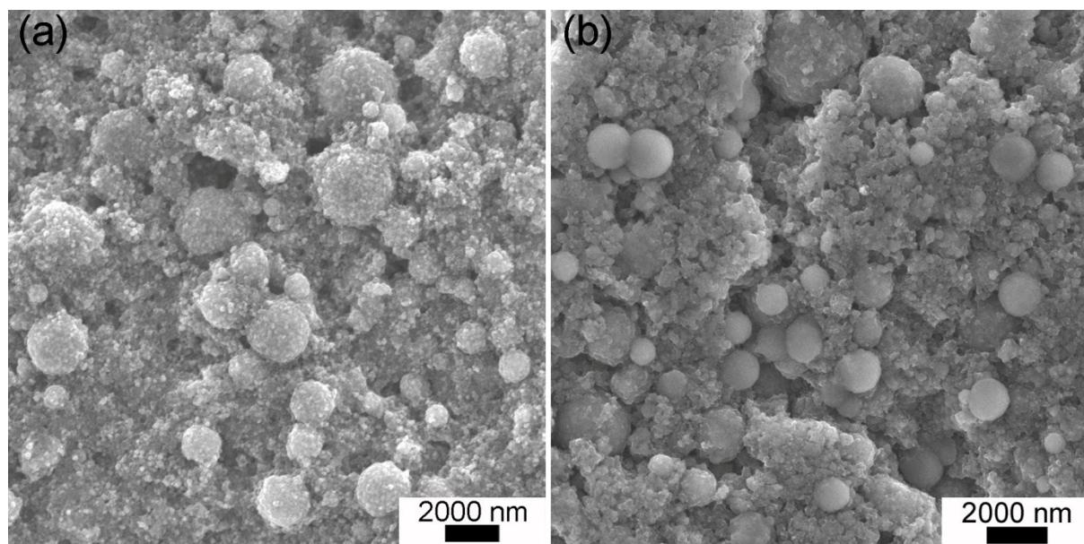
**Fig. S8** SEM images of electrode before cycling (a) and after 100 cycles at 400 mA g<sup>-1</sup> (b).
