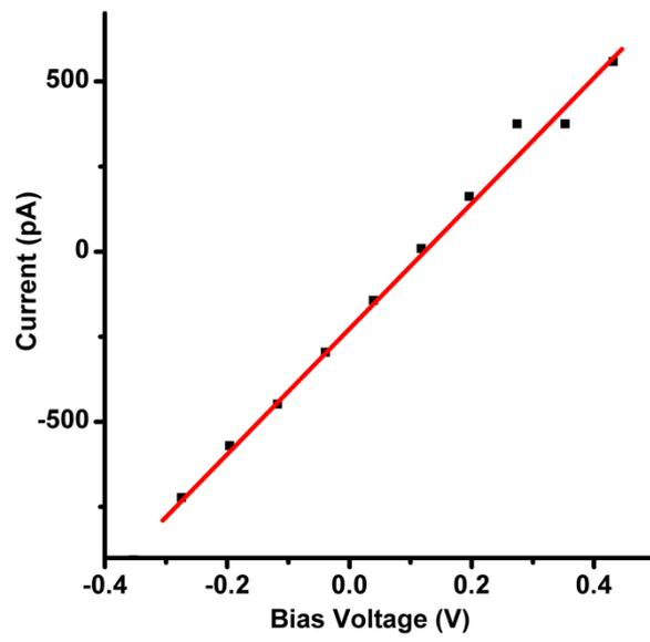
Figure S4. The  $I$ - $V$  curves of the contact between CAFM tip and bare  $\text{TiO}_2$
