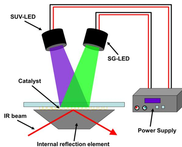
Figure S1. Scheme of the ATR-FTIR cell, including the SUV-LED and SG-LED
