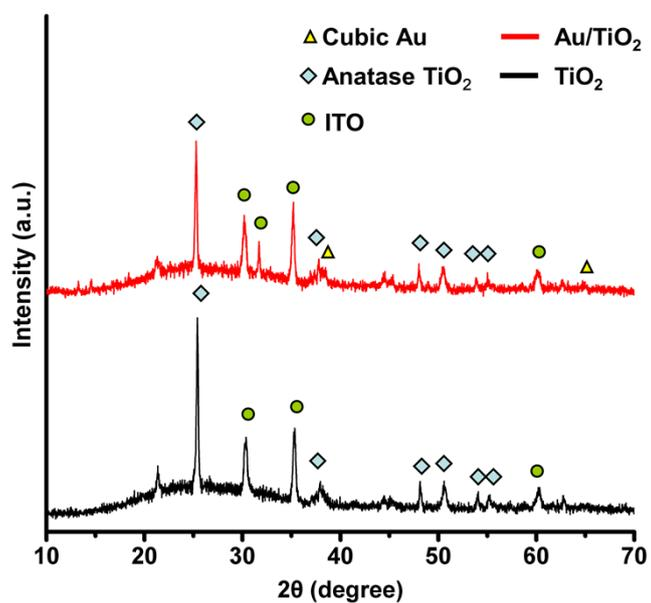
Figure S2. The X-ray diffraction patterns for TiO<sub>2</sub>, Au-TiO<sub>2</sub>. The plots are offset for clarity; peak positions for Au (Δ) and TiO<sub>2</sub> (◇), ITO (○) are indicated.
