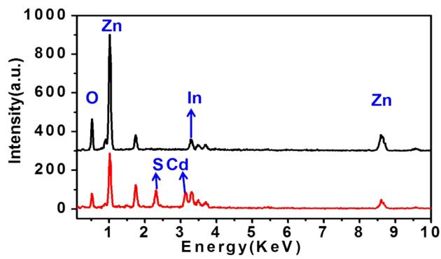
**Figure S1** EDX spectrum of pure ZnO nanorod array (upper) and CdS-coated ZnO nanorod array (bottom).
