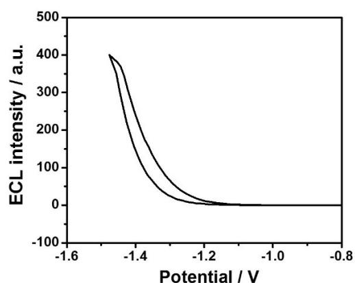
**Figure S2** ECL-potential curve of CdS QD modified electrode in 0.1 M PBS (pH 7.4) containing 0.1 M KCl and 0.05 M  $\text{K}_2\text{S}_2\text{O}_8$ . Scan rate is 100 mV s<sup>-1</sup> and the photomultiplier tube (PMT) voltage is set to be -800 V.
