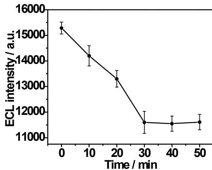
**Figure S7** Effect of incubation time on the ECL response of the immunosensor.
