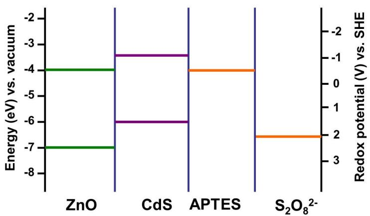
**Figure S5** The band levels of ZnO, CdS, APTES and  $\text{S}_2\text{O}_8^{2-}$ .
