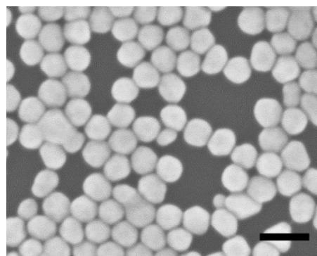
**Figure S6** SEM of gold nanoparticles. All the SEM images are taken using a field-emission scanning electron microscopy (FESEM, FEI Quanta 200F). The scale bar is 100 nm.
