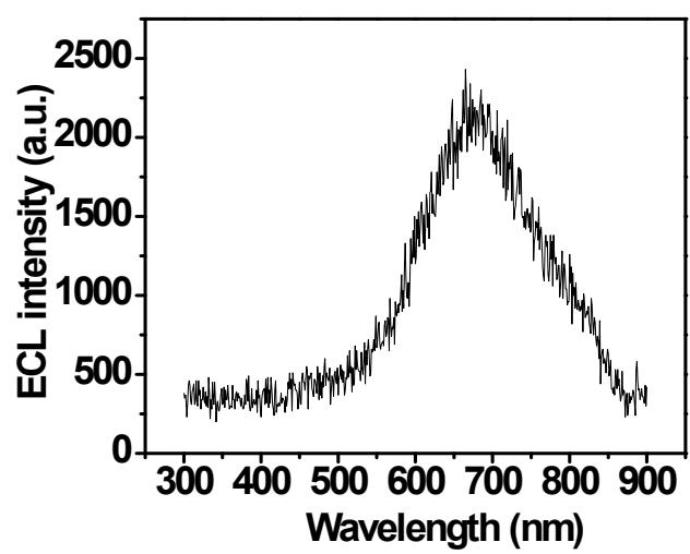
**Figure S3** ECL spectrum of Au/APTES/CdS-coated-ZnO modified electrode in 0.1 M PBS (pH 7.4) containing 0.1 M KCl and 0.05 M  $\text{K}_2\text{S}_2\text{O}_8$ .
