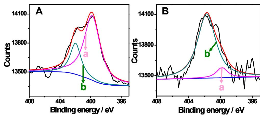
**Figure S4** XPS spectra of N 1s before (A) and after (B) the ECL process for 20 min.
