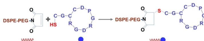
Figure S1. Schematic illustration of the conjunction of DSPE-PEG and cyclic RGD peptide.
