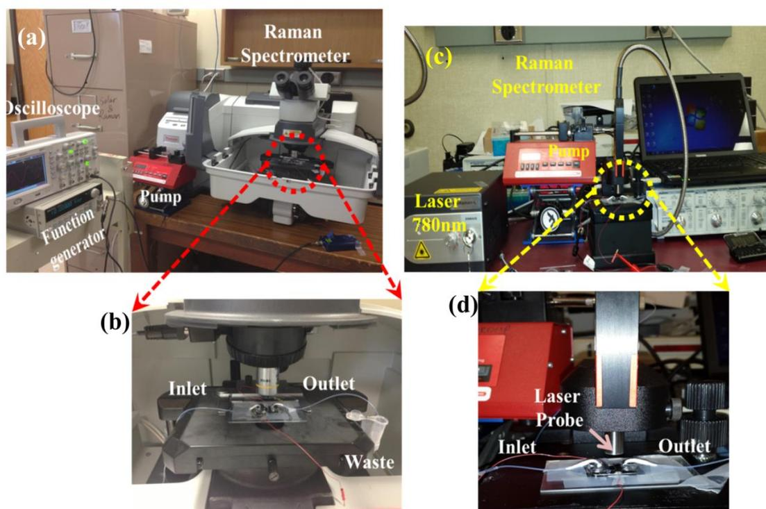
**Figure S1.** Experimental setup of Raman measurement on the DEP chip. (a) The confocal Raman microscope (DXR Raman spectrophotometer, Thermo Scientific) and (b) the microfluidic device under 10X objective of the Raman microscope. (c) The portable Raman Instrument (Pro Raman L, Enwave Optronics Inc.) and (d) is the alignment to the microfluidic device under 100  $\mu\text{m}$  probe.
