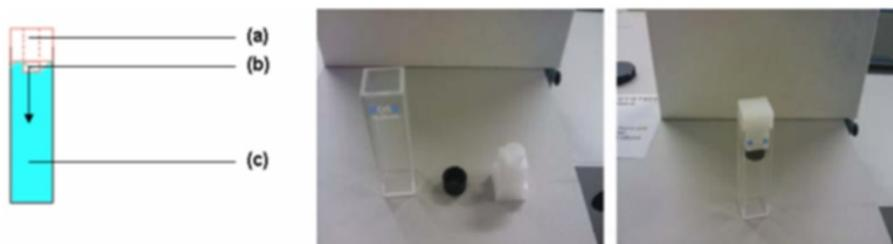
**Figure S5.** Custom made release experiment setup featuring a 200  $\mu\text{L}$  Teflon tube (a) which is closed by a dialysis membrane (b). This setup is put onto a fluorescence cuvette filled with the desired buffer (c).
