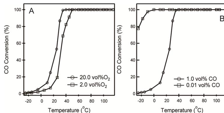
**Figure S2.** The effect of oxygen (A) and CO (B) concentration on the catalytic activity of 5.9 wt% Pd doped catalyst. (Catalyst: 200 mg; space velocity: 15000 ml h<sup>-1</sup> g<sup>-1</sup>. Feed gas: 1.0 vol% CO and desired O<sub>2</sub> balance with N<sub>2</sub> (A); 20.0 vol% O<sub>2</sub> and desired CO balance with N<sub>2</sub> (B).)
