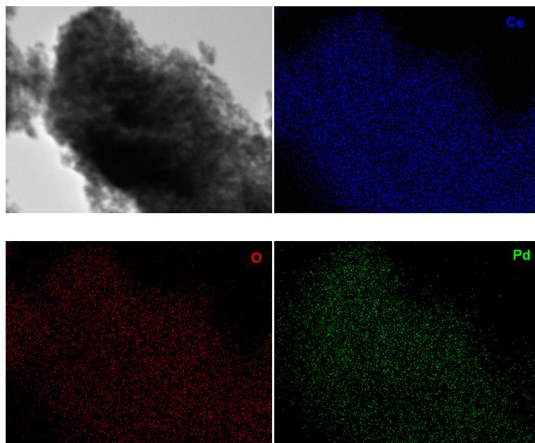
**Figure S1.** The EDX mapping of 5.9 wt% Pd doped catalyst.
