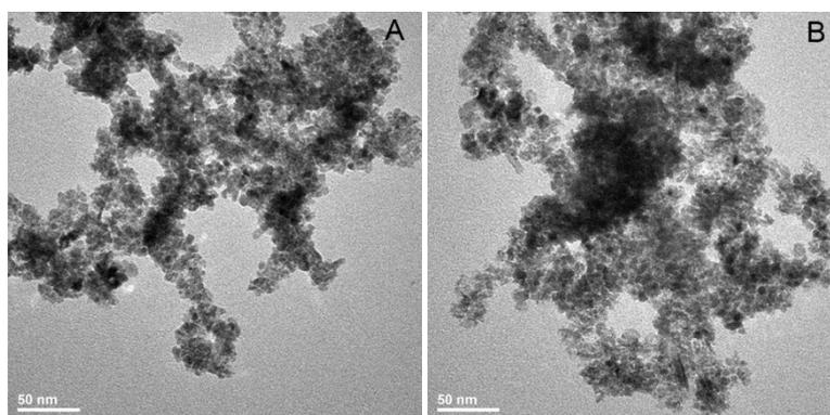
**Figure S6.** The TEM images of 5.9 wt% Pd-CeO<sub>x</sub> catalyst after reaction under dry (A) and moisture (B) condition.
