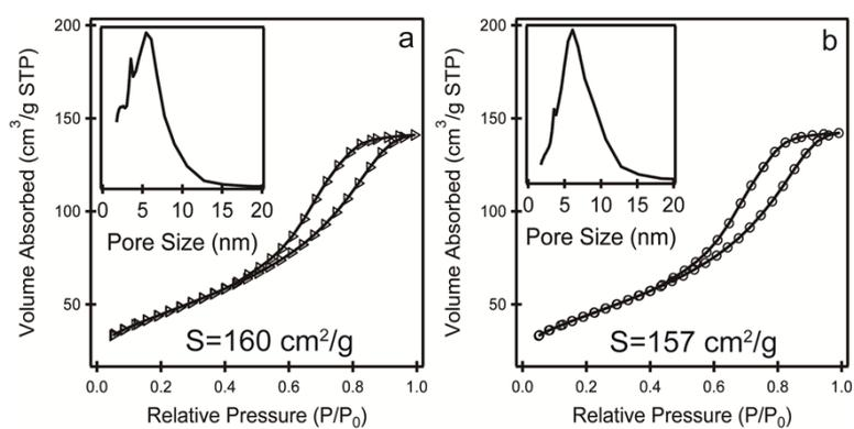
**Figure S5.** The N<sub>2</sub> adsorption-desorption isotherms of 5.9 wt% Pd-CeO<sub>x</sub> catalyst after reaction under dry (a) and moisture (b) condition.
