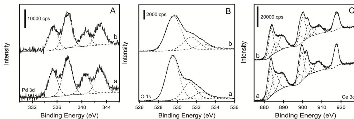
**Figure S7.** XPS spectra of Pd 3d (A), O 1s (B) and Ce 3d (C) of 5.9 wt% Pd-CeO<sub>x</sub> catalyst after reaction under dry (a) and moisture (b) condition.
