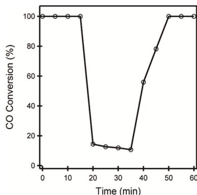
**Figure S3.** The effect of O<sub>2</sub> on the low temperature CO oxidation over 5.9 wt% Pd-CeO<sub>x</sub> catalyst at 35°C.
