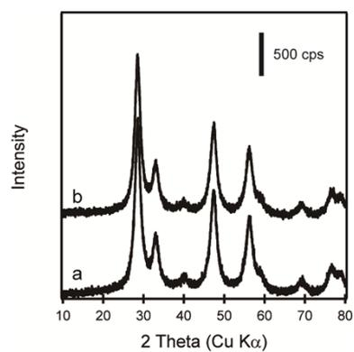
**Figure S4.** The XRD patterns of 5.9 wt% Pd-CeO<sub>x</sub> catalyst after reaction under dry (a) and moisture (b) condition.
