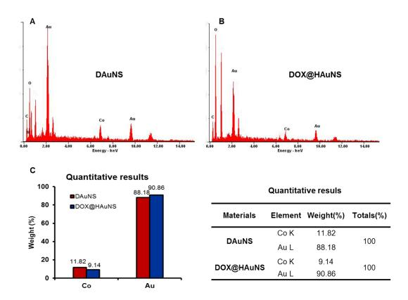
**Figure S6.** Analysis of metal contents by Energy dispersive X-ray (EDX). **(A)** EDX spectrum of DAuNS. **(B)** EDX spectrum of DOX@HAuNS. **(C)** Quantitatve results of DAuNS and DOX@HAuNS from A and B.
