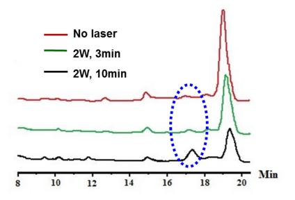
**Figure S7.** The stability of DOX under laser irradiation. After different time of laser irradiation, solution was detected with HPLC. Blue broken line circle indicates the increase of the peak height after the laser of 10 min (2.0 W/cm<sup>2</sup>).
