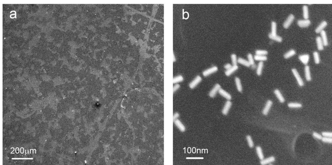
**Figure S1.** Scanning electron microscope (SEM) images of a) the as-grown 2H-MoS<sub>2</sub> on Si substrate and b) Ag@Au nanorattles. The dense MoS<sub>2</sub> samples ensure a high catalytic efficiency in hydrogen evolution reactions. The coupling between different Ag@Au nanorattles can be negligible for few clusters are formed, and thus keeps the resonance peak at 690nm.
