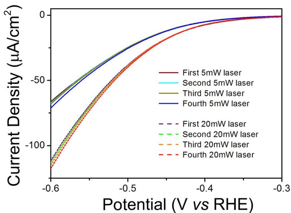
**Figure S5.** HER polarization curves under 690nm laser illumination, for MoS<sub>2</sub> monolayer with Ag@Au nanorattles. At a certain power, the phase transition gets saturated with the polarization curves keep similar at the first and fourth measurement.
