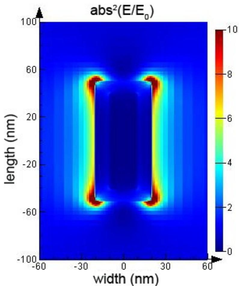
**Figure S4.** Calculated near-field optical intensity map of Ag@Ag nanorattles with a length of 100nm and width of 40nm by FDTD simulation.
