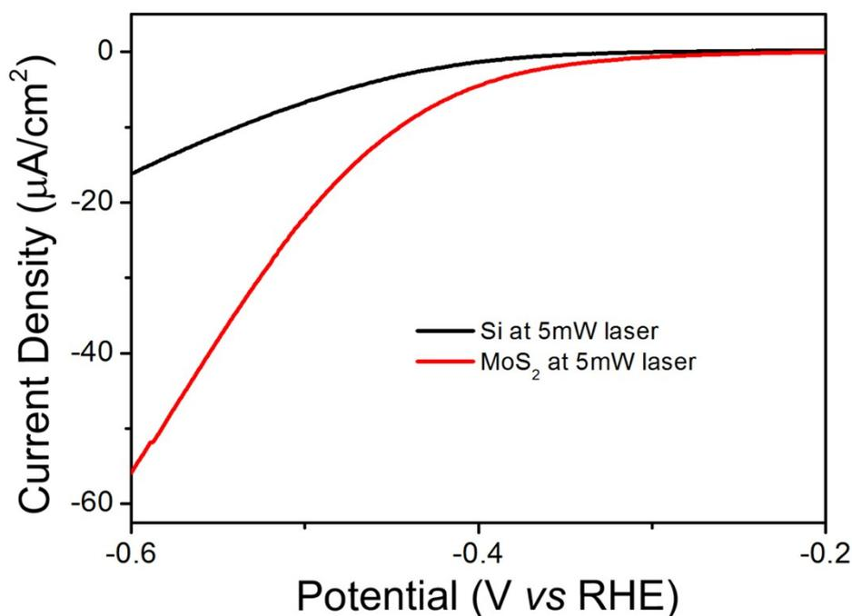
**Figure S3.** HER polarization curves under 690nm laser illumination, for Si and MoS<sub>2</sub>, respectively. Due to the imperfect conductivity of silicon, the HER performance is poor, but the catalytic performance of MoS<sub>2</sub> can be measurable.
