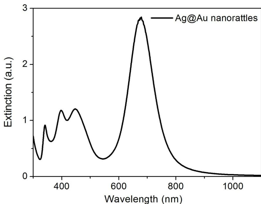
**Figure S2.** Extinction spectrum of Ag@Au nanorattles. The nanorattle exhibits both a longitudinal plasmon resonance at 690nm and a transverse mode around 420nm according to different incident laser polarization. These small peaks are the coupling modes. At 532nm, the Ag@Au nanorattles are off- resonant.
