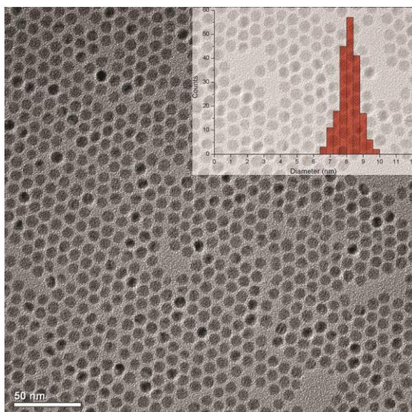
**Fig. S2.** Typical TEM image of the OA capped CdSe/CdS core/shell NCs, scale bar: 50 nm. The inset is the size histograms obtained from 200 particles in the image.
