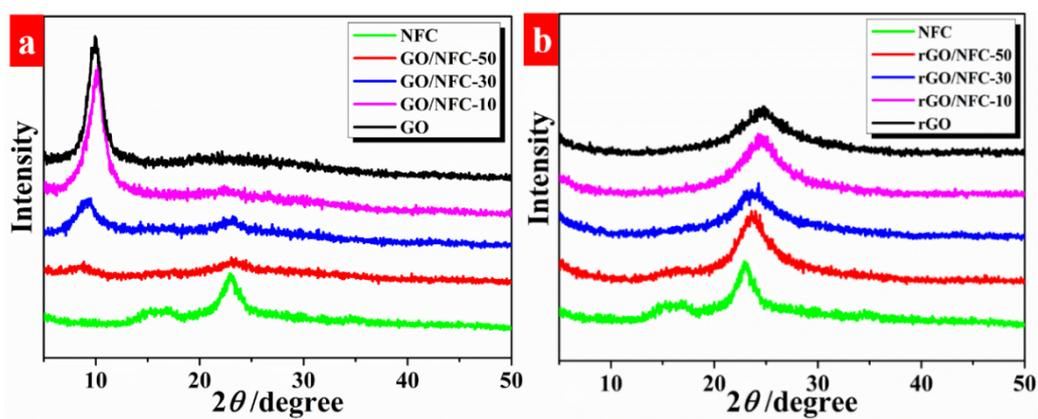
**Figure S4.** XRD pattern of (a) NFC, GO and GO/NFC, (b) NFC, rGO and rGO/NFC.
