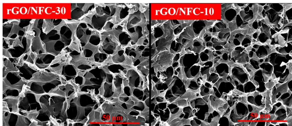
**Figure S3.** SEM images of rGO/NFC-30 and rGO/NFC-10 aerogels after hydroiodic acids reduction and freeze-drying.
