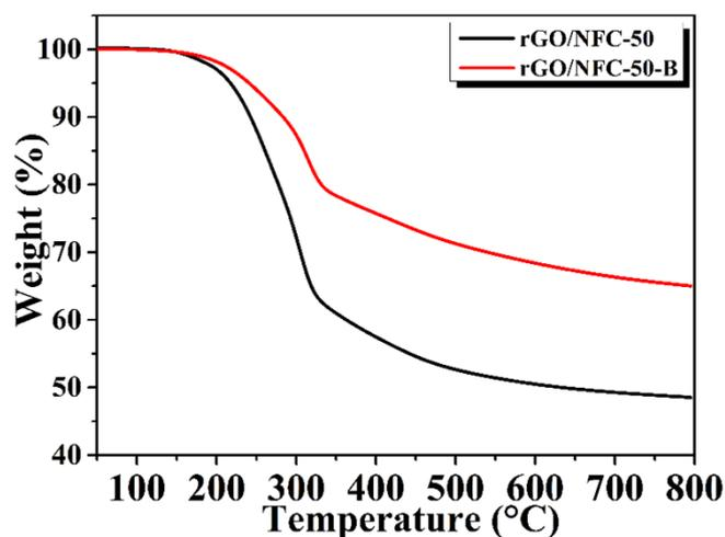
**Figure S10.** Thermo gravimetric analysis of rGO/NFC-50 aerogel in nitrogen before (rGO/NFC-50, black curve) and after (rGO/NFC-50-B, red curve) being recycled for five times sorption-combustion process.
