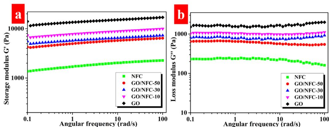
**Figure S2.** Dynamic properties of the GO/NFC hydrogels: dynamic frequency sweep (25°C) of the gels at a strain rate of 0.5%. a) storage modulus plots, b) loss modulus plots.
