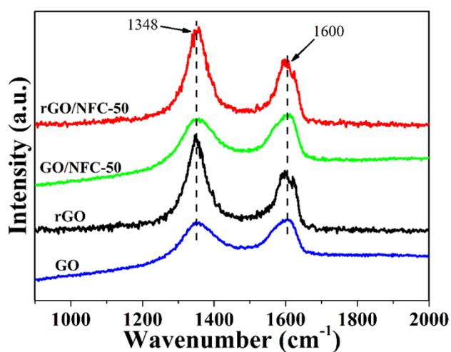
**Figure S5.** Raman spectra of GO, rGO, GO/NFC-50 and rGO/NFC-50 aerogels.
