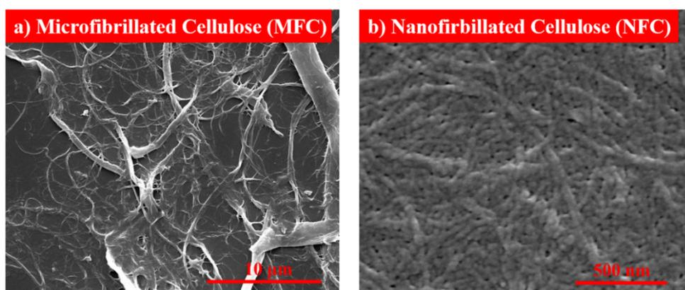
**Figure S1.** SEM images of original microfibrillated cellulose (a) and after TEMPO-oxidation (b).
