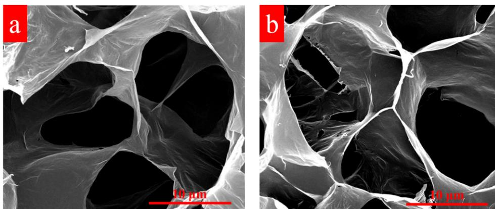
**Figure S7.** SEM images of the rGO/NFC-50 aerogel before (a) and after fatigue cyclic compression test (50 cycles, b), indicating that there are no obvious structural changes.
