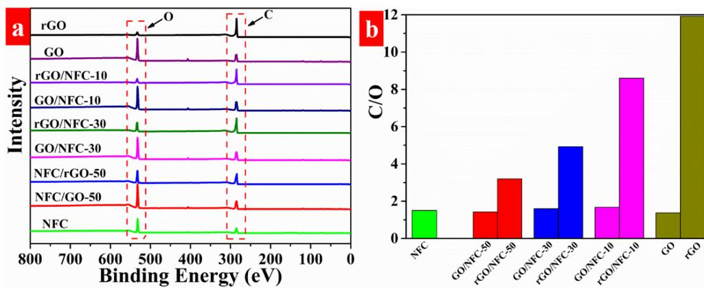
**Figure S6.** XPS spectra (a) and variation of the C/O atomic ratio (b) of the neat NFC aerogel and hybrid aerogels of before and after reduction by hydroiodic acids.
