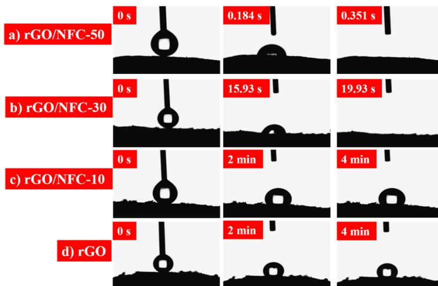
**Figure S8.** Photographs of a water droplet absorbed by (a) rGO/NFC-50 and (b) rGO/NFC-30 aerogel. Photographs of a water droplet supported on (c) rGO/NFC-10 and (d) rGO aerogel.
