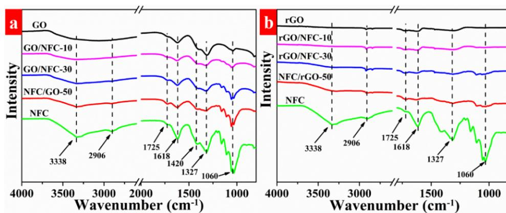
**Figure S9.** FT-IR spectra of the original NFC aerogel and GO, rGO, hybrid aerogels of before (a) and after (b) reduction by hydroiodic acids.
