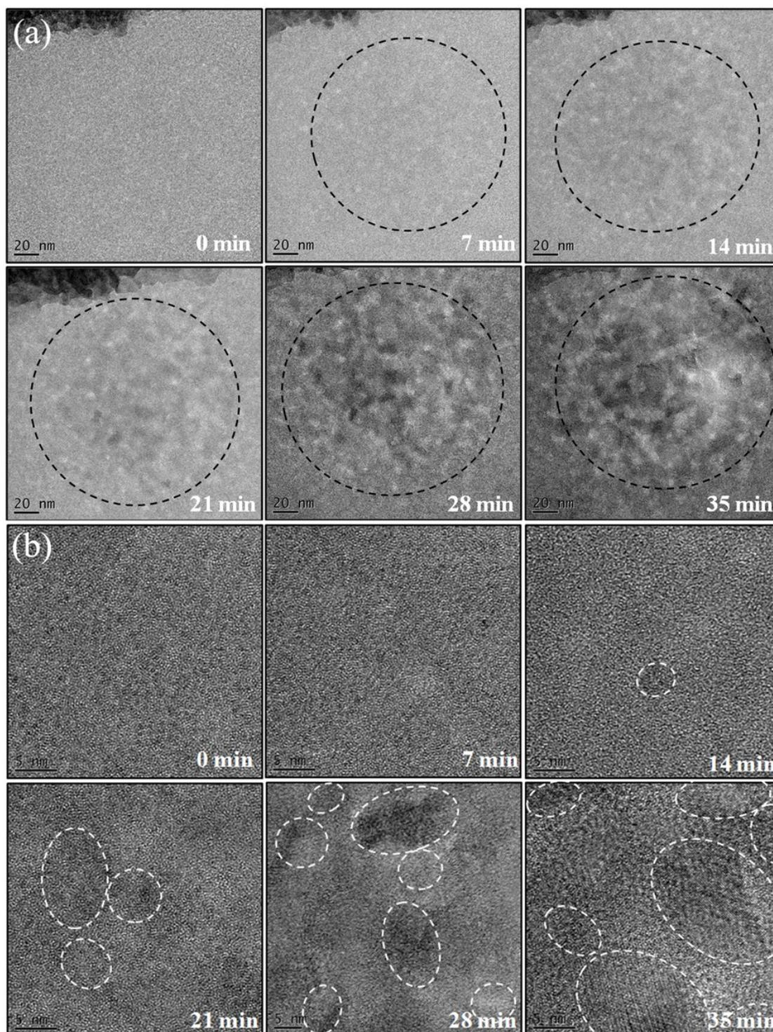
**Figure S2** *In-situ* crystallization of  $\text{Ge}_2\text{Sb}_2\text{Te}_5$  film by electron-beam irradiation, characterized by FEI Tecnai F20 TEM at 200 KeV in (a) TEM and (b) HRTEM modes. The diameter of beam spot is about 180 nm. To insure that the same area ( $a_{ei}$ ) is irradiated by the high-energy electrons, marked by black dashed circle in the figure,
