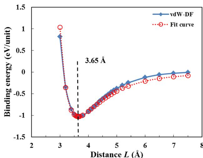
Figure S1: Interlayer binding energy ( $E_b$ ) of COF-1 (AA stacking) as a function of interlayer distance  $L$  in the range of 2.0-7.5 Å. Black dotted line represents an equilibrium interlayer distance,  $\sim 3.65$  Å.
