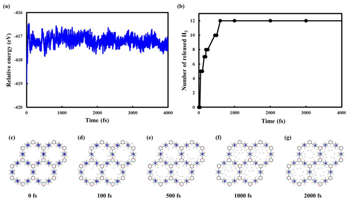
Figure S9: Molecular dynamics for hydrogen release process in CaCOF-1 at  $4.3 \text{ \AA}$  at room temperature (300 K). (a) Relative energy of  $12\text{H}_2$  on CaCOF-1 in unit cell as a function of time; (b) Number of released hydrogen in unit cell as a function of time; (c)-(g) Top view of  $\text{H}_2$ -CaCOF-1 at 0, 100, 500, 1000, and 2000 fs, respectively.
