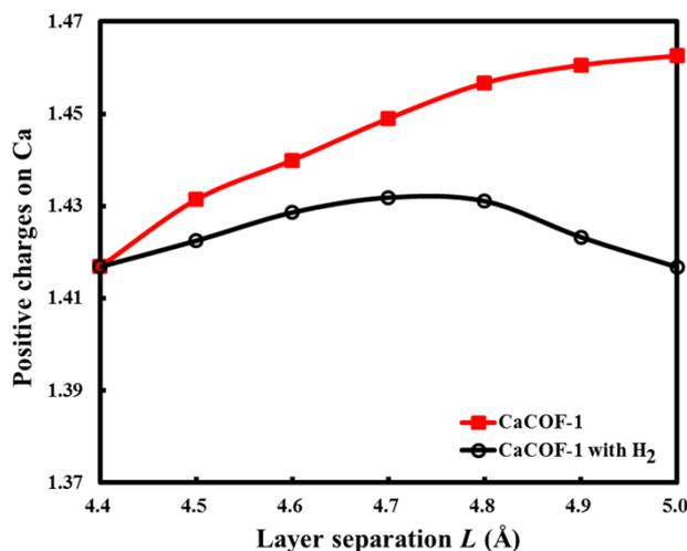
Figure S5 Positive charges on Ca atoms in clean and hydrogen adsorbed CaCOF-1 as a function of layer separation.
