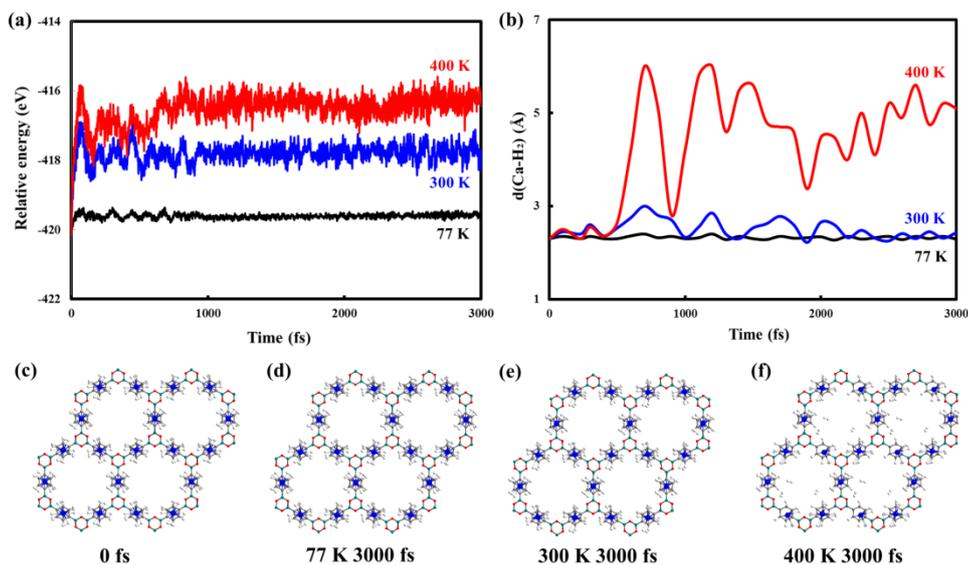
Figure S8: Molecular dynamics for hydrogen storage in CaCOF-1 at 4.8 Å at three different temperatures (77, 300 and 400 K). (a) Relative energy of  $12\text{H}_2$  on CaCOF-1 in unit cell as a function of time. (b) Distance between Ca and one of adsorbed  $\text{H}_2$  molecules on CaCOF-1 ( $d(\text{Ca}-\text{H}_2)$ ) as a function of time. (c)-(f) Top view of  $\text{H}_2$ -CaCOF-1 at 0 fs and 3000 fs at 77, 300, 400 K, respectively.
