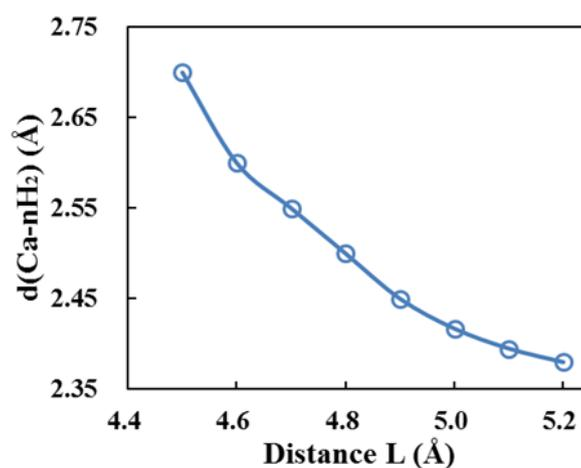
Figure S6: Average distance between Ca and adsorbed H<sub>2</sub> molecules on CaCOF-1 ( $d(\text{Ca-nH}_2)$ ) as a function of interlayer distance  $L$ . With the distance  $L$  increasing,  $d(\text{Ca-nH}_2)$  is getting small that shows a stronger interaction.
