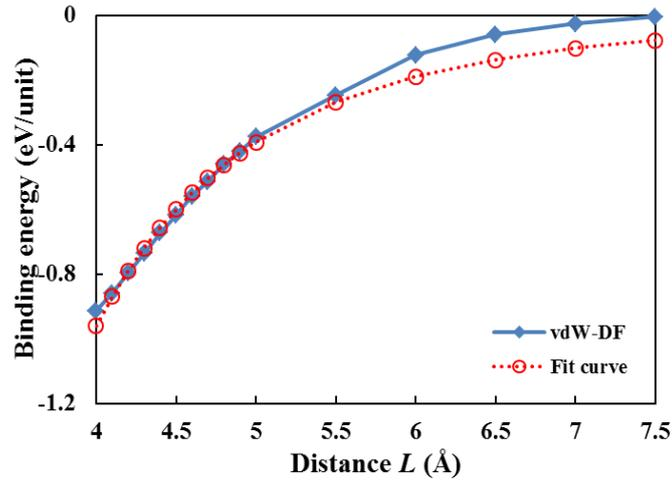
Figure S2: Interlayer binding energy of COF-1 (AA stacking) as a function of interlayer distance  $L$  in the range of 4.0-7.5 Å.
