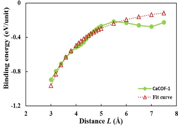
Figure S3: Interlayer binding energy of CaCOF-1 as a function of interlayer distance  $L$ .  $E_b$  (CaCOF-1) is obtained:  $E_b$  (CaCOF-1) =  $E_{vdW-DF} - E_{GGA}$ .
