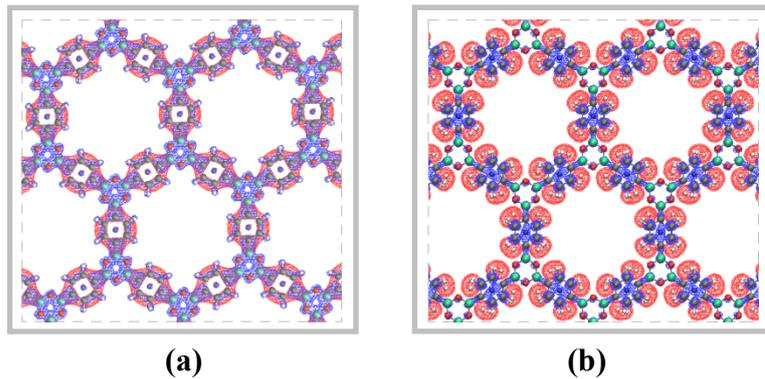
Figure S4: (a) Charge density difference in CaCOF-1 upon Ca adsorption. (b) Charge density difference in CaCOF-1 upon H<sub>2</sub> adsorption. Red and blue clouds correspond to electron depletion and accumulation regions upon Ca binding (a) and H<sub>2</sub> binding (b), respectively.
