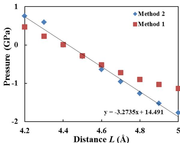
Figure S7: Pressure as a function of interlayer distance  $L$ . The method 1 is to get the pressure directly by VASP and method 2 [5] means to obtain the pressure by formula, namely,  $P(V) = -dE(V)/dV$ .
