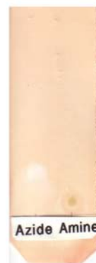
Fig. 2 TLC analysis of a diazide (Table 1, Entry 10), eluted with ethyl acetate/cyclohexane (1/5) and an amine (1,8-diaminooctane). The TLC plate was developed with the "click-staining-reagent". It shows the different staining of azides (left spot) and amines (right spot) which allows their differentiation.
