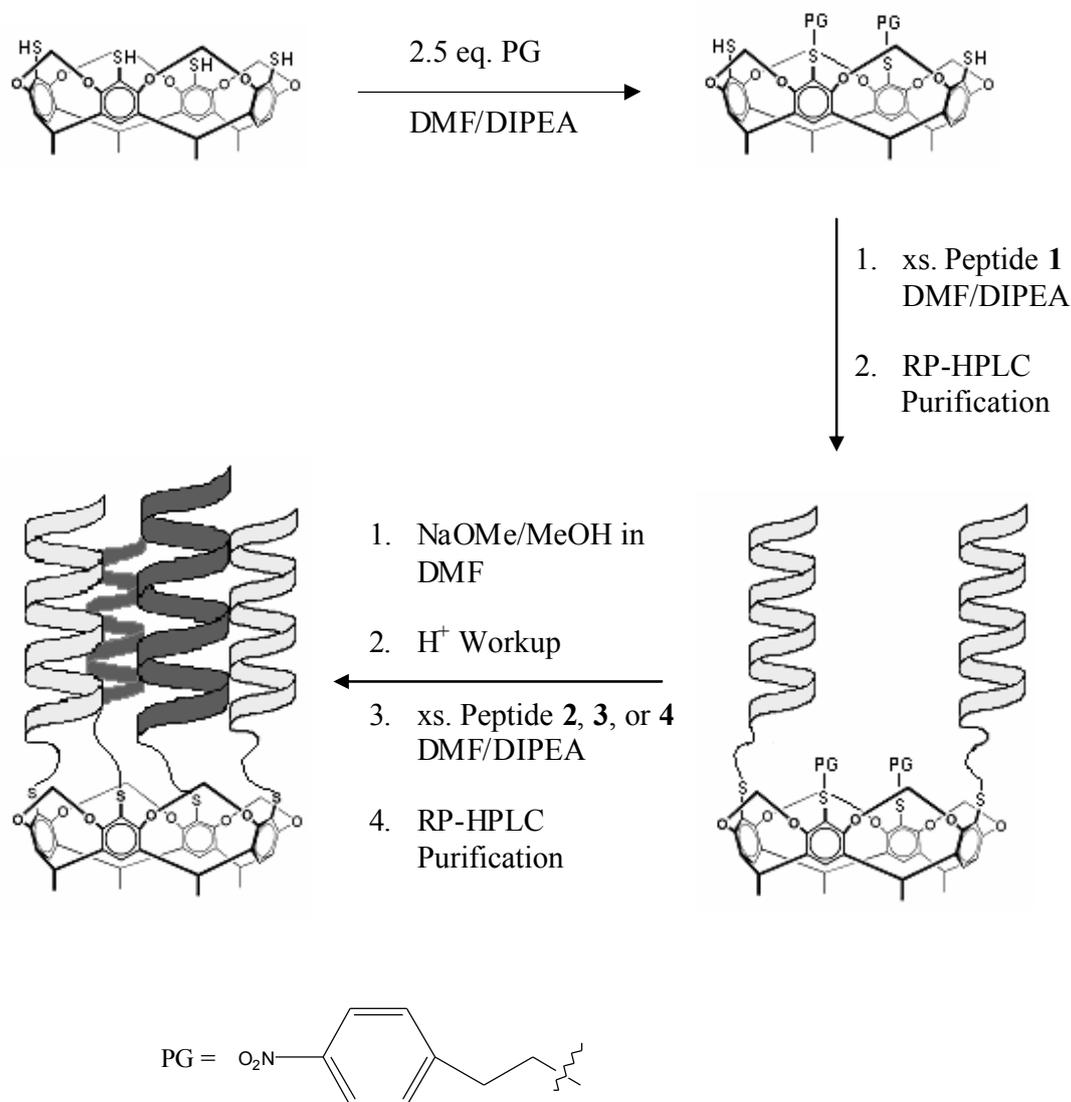
**Figure 19.** Schematic Representation Outlining the General Synthesis for an a,c Hetero- TASP where PG is the 2-(4-nitrophenyl)ethyl Group.
