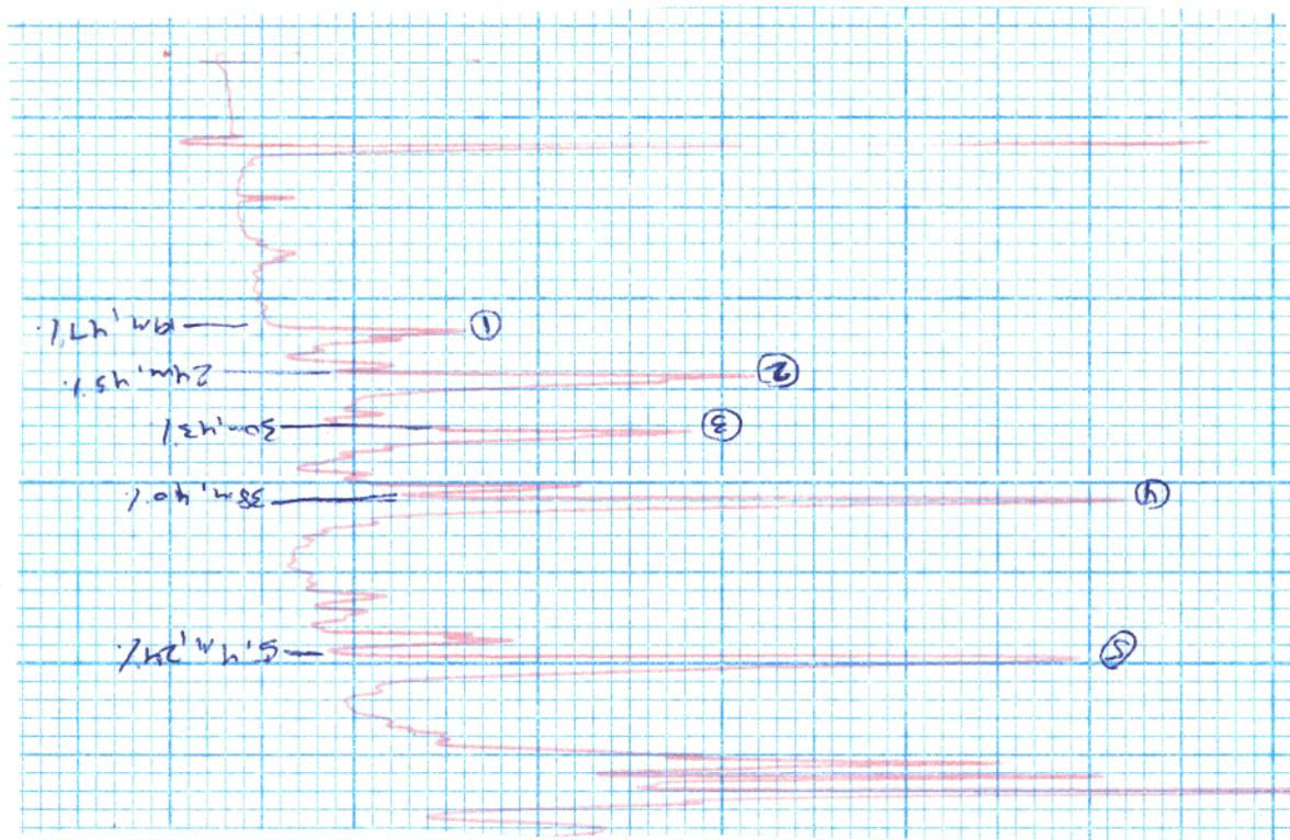
**Figure 20.** The Purification of the Crude Reaction Mixture of the Ig3 Substituted Hetero-TASPs by Preparatory Reversed-Phase HPLC Using a Gradient of 20-70 % Acetonitrile (with 0.05 % TFA) in Water (with 0.1 % TFA) Over 60 Minutes.
