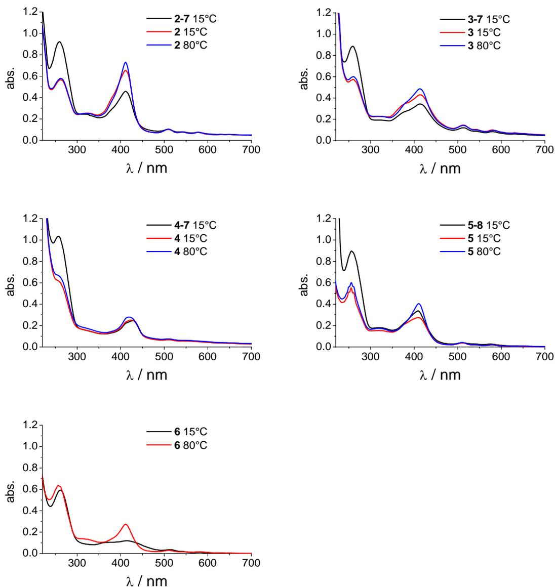
**FigS2:** UV-vis spectra of the porphyrin-DNA strands as single strands at 15°C and 80°C, and as double strands at 15°C (exc. **6**: single strand only).
