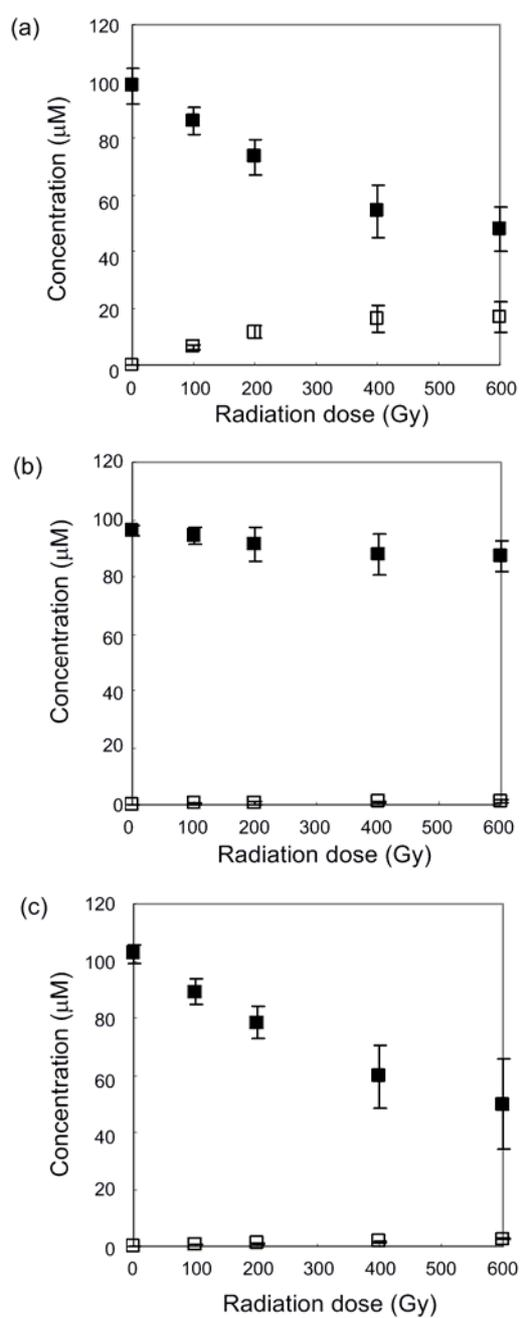
**Fig. S1.** Radiolytic reduction of 100 μM **oxo-ara-C** (closed square) to release **ara-C** (open square)
